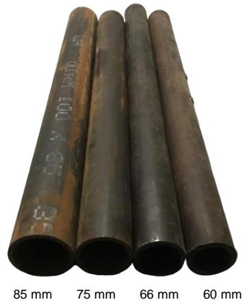
Figure 2.5 – Steel calibration tubes of internal diameter 60 mm, 66 mm, 75 mm and 85 mm
