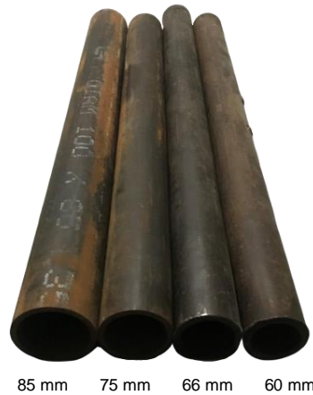
Figure 2.5 – Steel calibration tubes of internal diameter 60 mm, 66 mm, 75 mm and 85 mm
