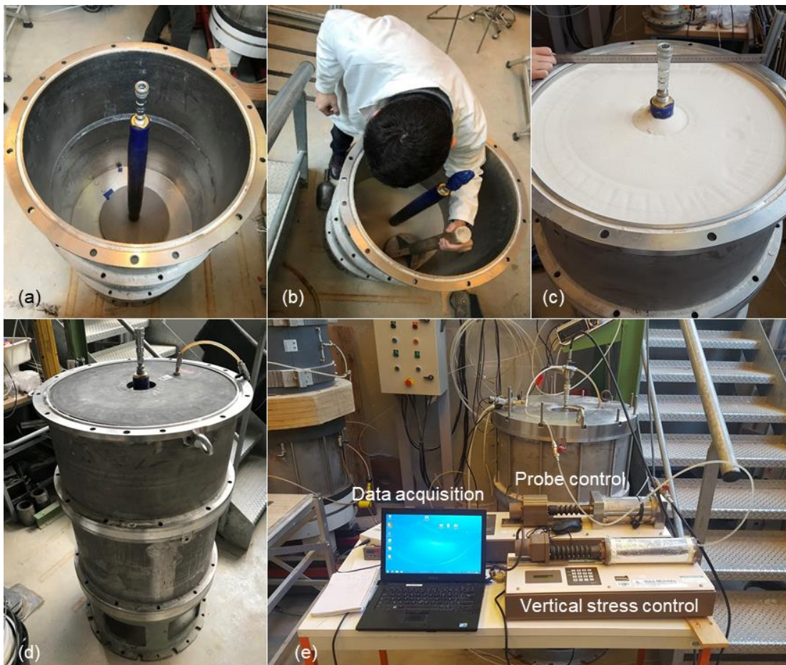
Figure 2.26 – (a) Probe inside KCC, (b) manual compaction of 10 cm sand layer, (c) end of compaction, (d) installation of the pressurization cushion, (e) fully assembled set up.
