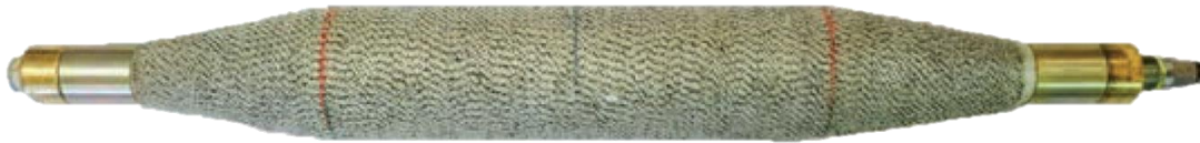
Figure A.19 – External textile restraining sheath employed in FC 60 probe THP (2015)
