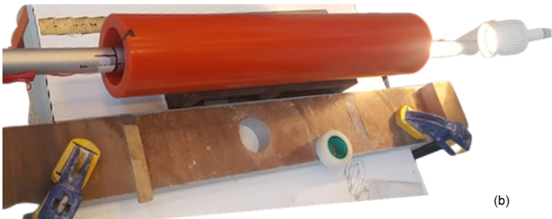
Figure 2.8 – Metallic rod inserted into the PU cylinder and strain gauge fully glued
