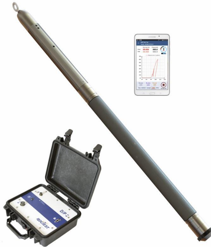
Figure A.25 – DMP 95 mm dilatometric probe. Radial strains are assessed through induction sensors connected to metallic insertions trespassing the membrane. TELEMAC (2018)
