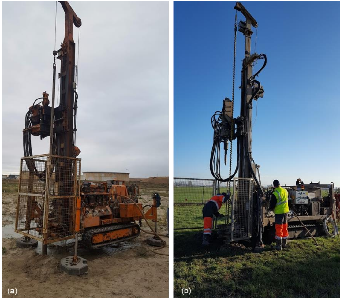
Figure 3.3 – Drilling rigs used: (a) Dunkirk testing site; (b) Merville testing site
