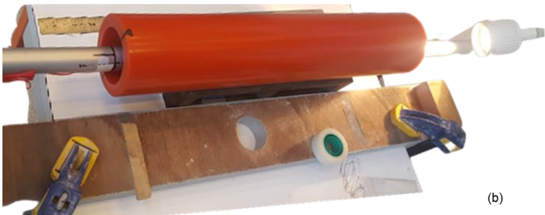
Figure 2.8 – Metallic rod inserted into the PU cylinder and strain gauge fully glued
