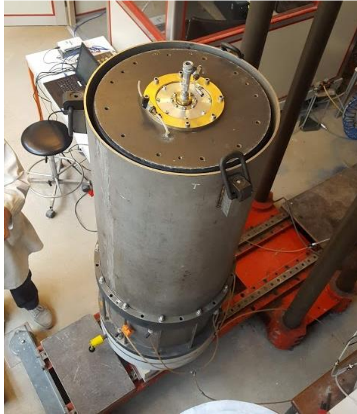
Figure 2.33 – External cylindrical enclosure set-up and detail of the empty space between the specimen and the enclosure, used for horizontal pressurization.
