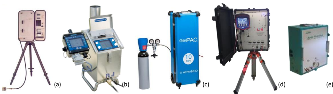
Figure A.6 – Examples of automatic control units. (a) PAC Baud (1985), (b) PREVO LUTZ (n.d.), (c) GeoPAC APAGEO (2017), (d) PresioLIM AUTO LIM (n.d.), (e) Auto-Pression Logic (2019)
