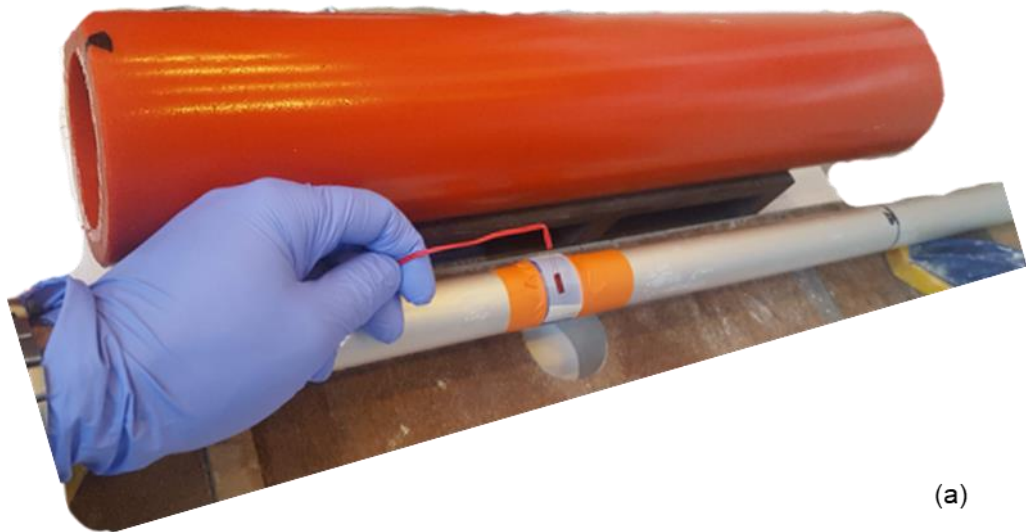
Figure 2.7 – Placing the strain gauge over the temporary support before applying glue
