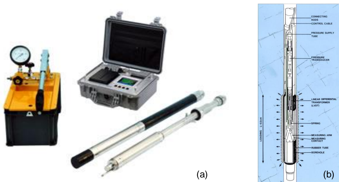
Figure A.14 – (a) OYO Elastmeter monocell pressuremeter probe for high-pressure applications (up to 20 MPa). Radial displacement transducers used to assess radial strain. (b) Probe scheme showing the displacement transducers OYO (2019c), (2019d)
