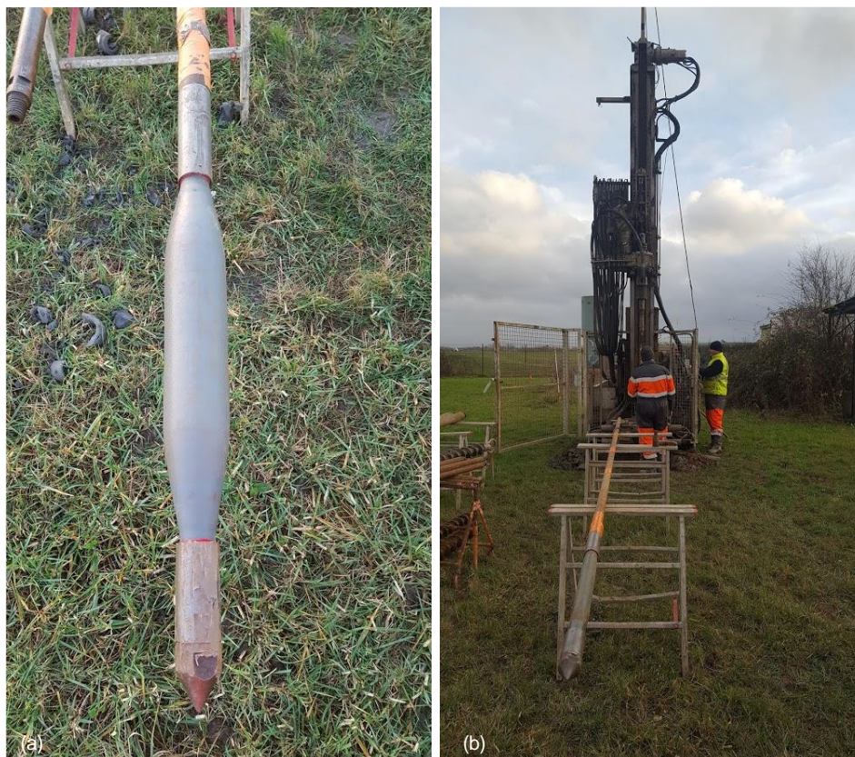
Figure 3.8 – (a) Photo of the probe assembled for the tests at Merville site; (b) view of the probe connected to the steel rods prior to its insertion into the ground
