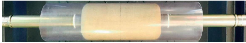
Figure A.20 – Textile sheath applied to the central measuring cell in FC 60 probe, imposing its cylindrical geometry THP (2015)
