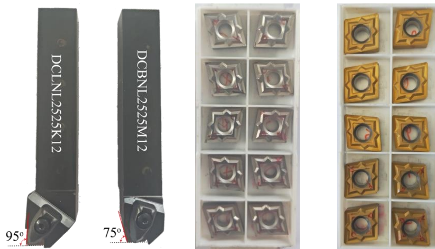
Fig. 100: Tool holders and inserts used in turning of Ti-6Al-4V alloy.
