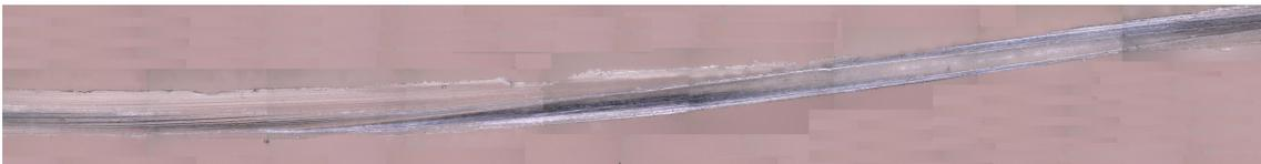
Figure B.4: An epoxy fibre. The fibre is twisted along the length due to the twists given to the teflon wires for consolidation.
