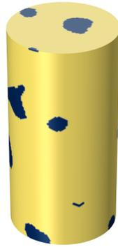
Figure 3: Virtually sampled cylindrical specimen of diameter 10 cm and height 20 cm, from the rock salt block shown in Figure 2.
