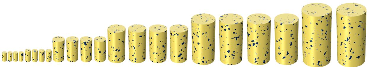
Figure 13: Virtual sampling of cylindrical specimens with a slenderness ratio of 2 from the block in Figure 2. From left to right, four specimens are cored having the diameters of  $4a$ ,  $5a$ ,  $10a$ ,  $15a$ ,  $20a$  and  $25a$ , with  $a$  the characteristic size of the heterogeneities.
