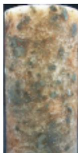
Figure 1: An example of a rock salt specimen tested at Mines ParisTech, with visible inclusions of insoluble materials.
