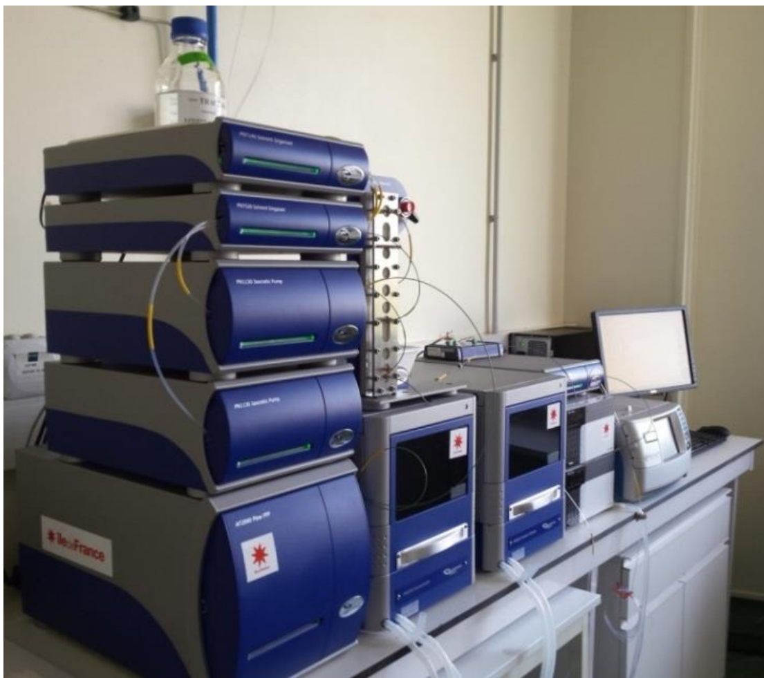
Figure 31. AF4-UV-DRI-MALS system used in this work
