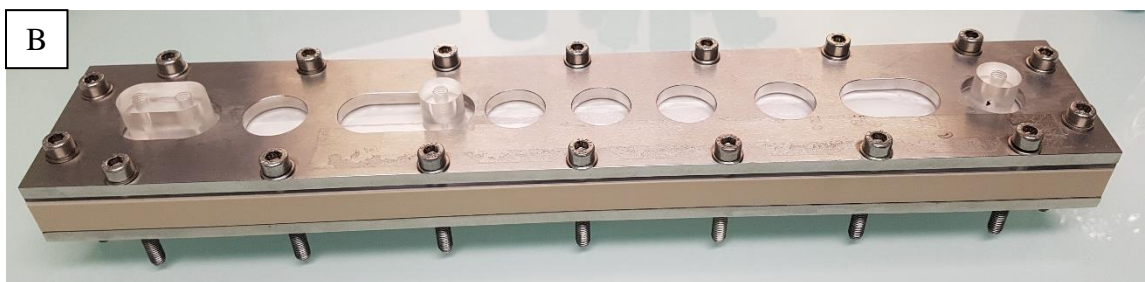
Figure 69. Different channel prototypes adapted to optical sensor measurements.
