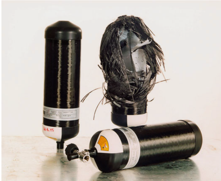
Figure 5.1: Examined breathing air cylinder of type IV from CFRP with PE-liner for a nominal working pressure of 300 bar (Taken from [86] Chapter 4.2. Experience with artificial ageing)
