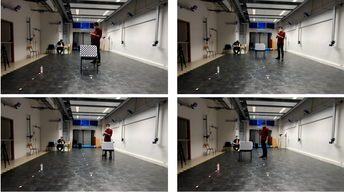
FIGURE 3.6: Calibration of the marker-less motion capture system: Placement of the calibration device at four different positions.
