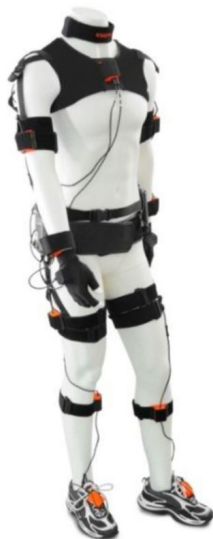
FIGURE 1.9: Placement of IMU sensors on the human body. Reproduced from Xsens.
