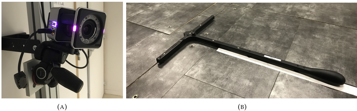
FIGURE 3.2: (A) Vicon Vero v1.3 camera (B) Vicon calibration device placed on the floor to set the global coordinate system of the Vicon system.
