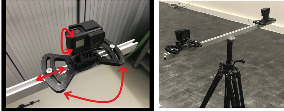
FIGURE 3.3: Left: the GoPro Hero 7 Black camera is mounted on the aluminum bar using the 3D printed fastening. The camera's position and orientation can be adjusted by the three degrees of freedom. Right: two cameras are mounted on the aluminum bar, which is installed on a tripod.
