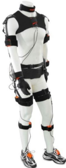
FIGURE 1.9: Placement of IMU sensors on the human body. Reproduced from Xsens.
