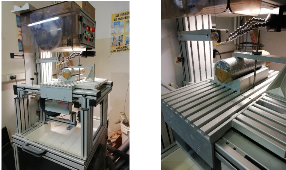
Fig. 2.3. The sawing machine with a core installed: far view (left) and near view (right)
