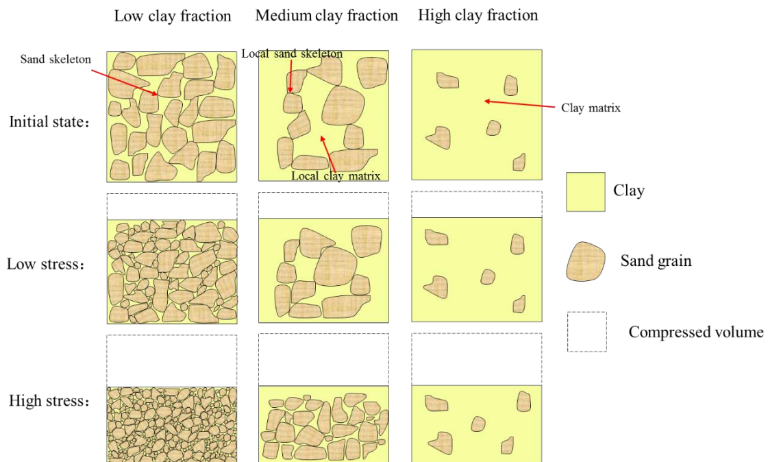
Fig. 4.11. Representation of soil structure changes during the compression process for different clay fractions
