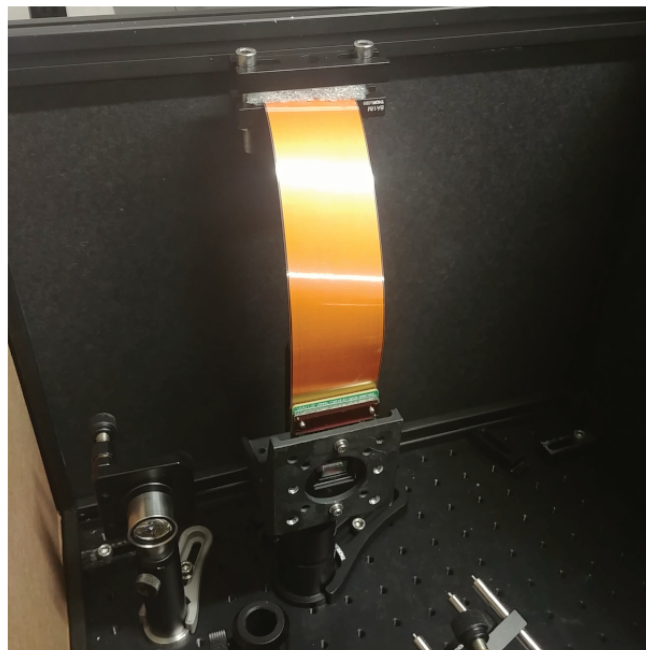
Figure A.1: Method used to dampen the vibrations of the DMD. The rigid orange ribbon cable is attached with foam and clamps in the top of the image.
