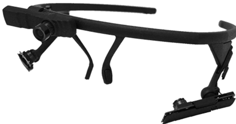
FIGURE 6.10 – Lunettes d'eye-tracking Pupil Core de PUPIL LABS [ Pupil Core ]
