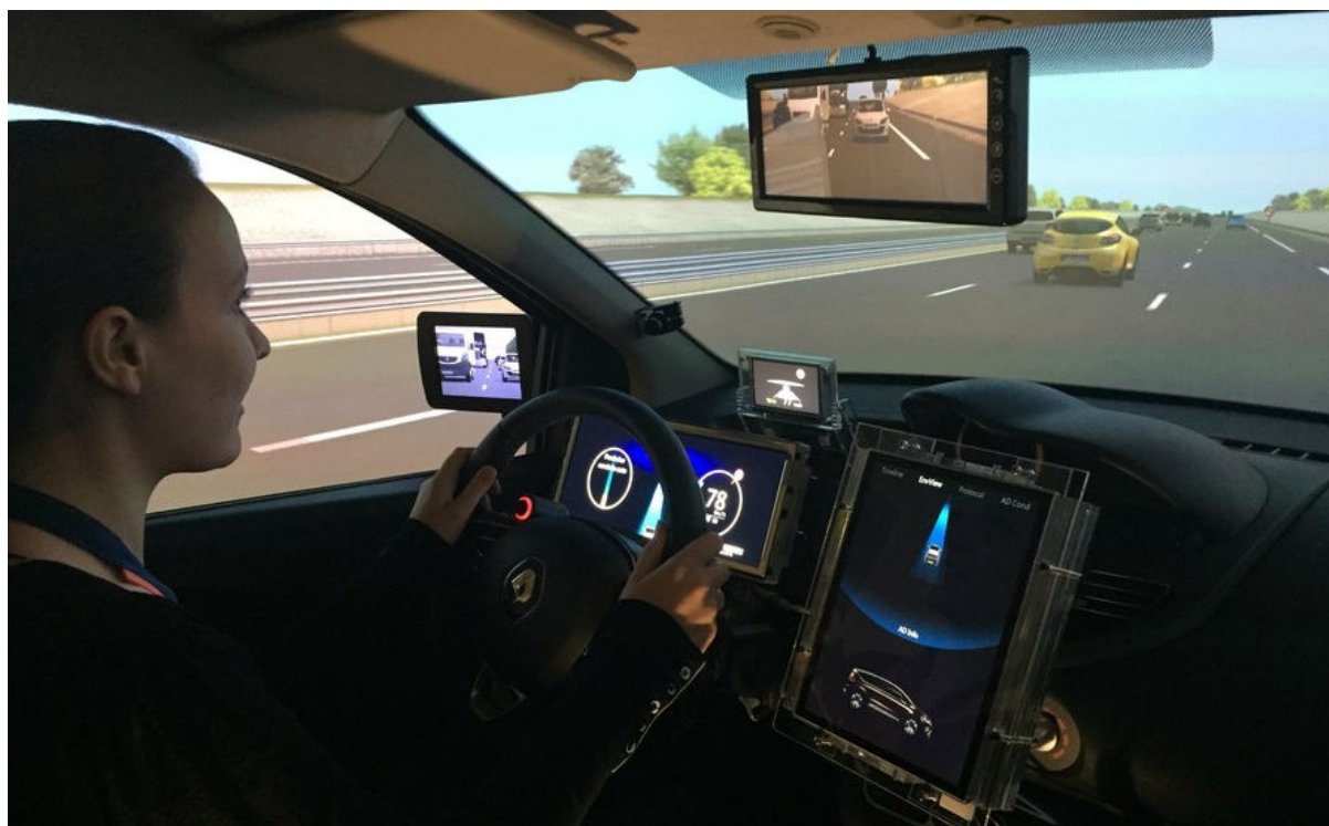
FIGURE 1.8 – Exemple de simulation driver in the loop
