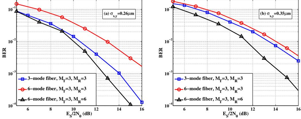
**Figure 2.21:** Performance of 3-mode fiber and 6-mode fiber using  $M_T$  transmit modes and  $M_R$  receiver side modes,  $SE = 6\text{bits/s}$
