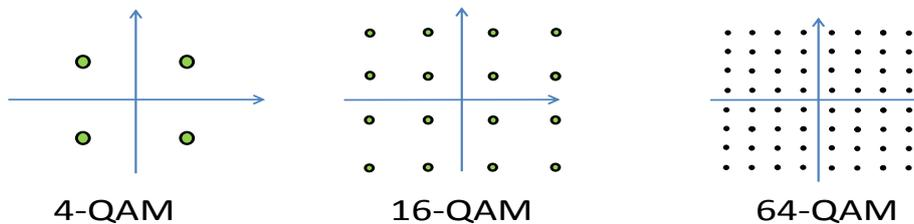
Figure 1.9: Constellations of 4-QAM, 16-QAM and 64-QAM.
