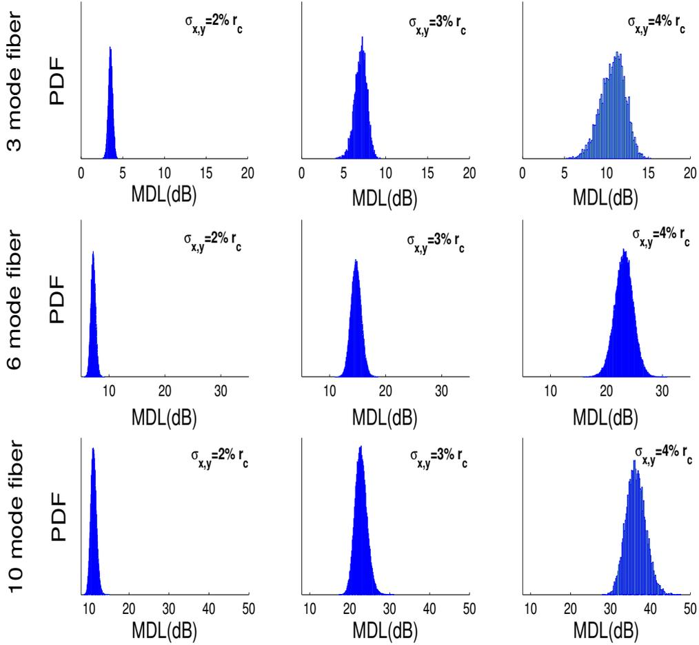
**Figure 2.5:** Probability distribution functions of MDL for 3, 6 and 10 mode fibers for different misalignment standard deviation  $\sigma_{x,y}$ .
