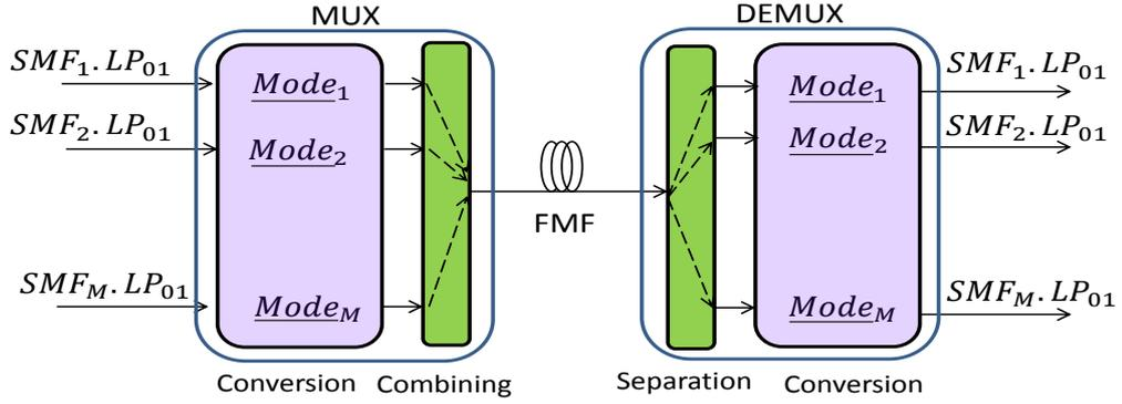
Figure 1.18: mode multiplexer and mode demultiplexer scheme
