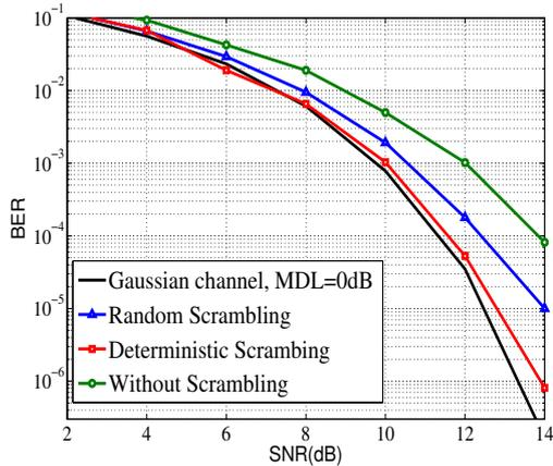
**Figure 2.16:** BER performance of 6-mode fiber,  $\sigma_{x,y} = 3\%r_c$
