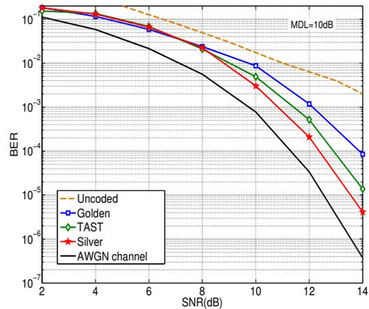
**Figure 3.4:** 2-modes fiber. BER versus SNR for the  $2 \times 2$  {Silver, Golden, TAST} codes, for MDL = 10 dB.
