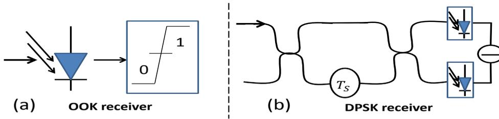
**Figure 1.10:** Direct detection receiver architecture : a) for NRZ-OOK format, b) for DPSK format.
