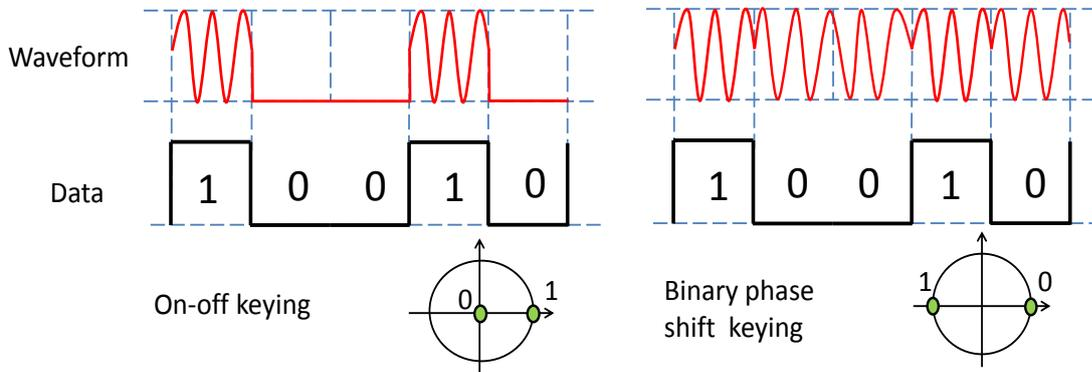
**Figure 1.8:** Modulated optical signal according to binary data: left OOK, right BPSK.
