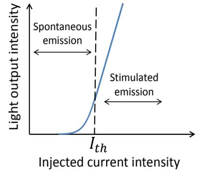
**Figure 1.5:** Laser intensity vs electrical input intensity.
