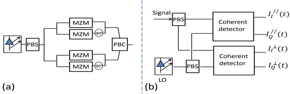
**Figure 1.13:** (a): PDM transmitter, (b): PDM coherent receiver
