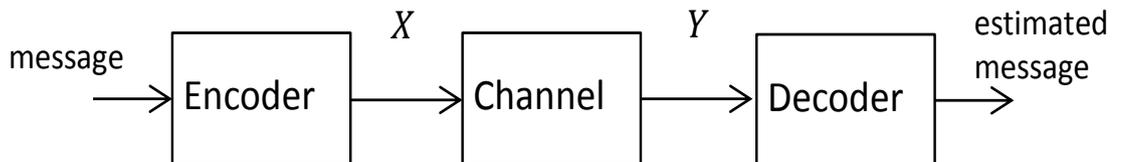
**Figure 2.1:** General communication channel including encoder and decoder.
