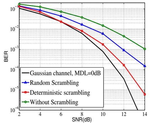
**Figure 2.17:** BER performance of 6-mode fiber,  $\sigma_{x,y} = 4\%r_c$
