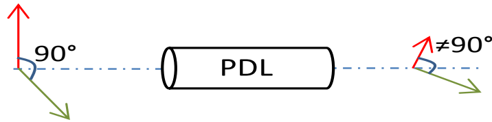
Figure 1.15: Loss of orthogonality and power imbalance due to PDL.
