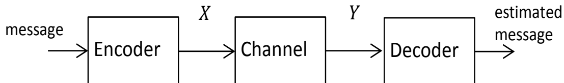
Figure 2.1: General communication channel including encoder and decoder.
