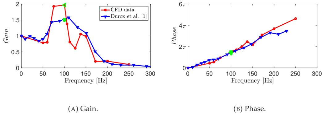
FIGURE 2.16: Gain and phase difference between velocity and flame surface area fluctuation of the ICF as a function of the incoming forcing frequency. The results for experiment [10] and CFD are compared. Also, the values for the gain and phase at 100 Hz for different mesh adaption temperature gradients are given for the following gradients; 10 K/m ( $\square$ ), 25 K/m ( $\circ$ ), 50 K/m ( $\triangleleft$ ) and 100 K/m ( $\triangle$ ).
