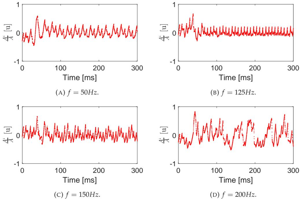
FIGURE 2.13: Flame surface area fluctuation due to four different incoming forcing frequencies, underscoring the flame different responses.
