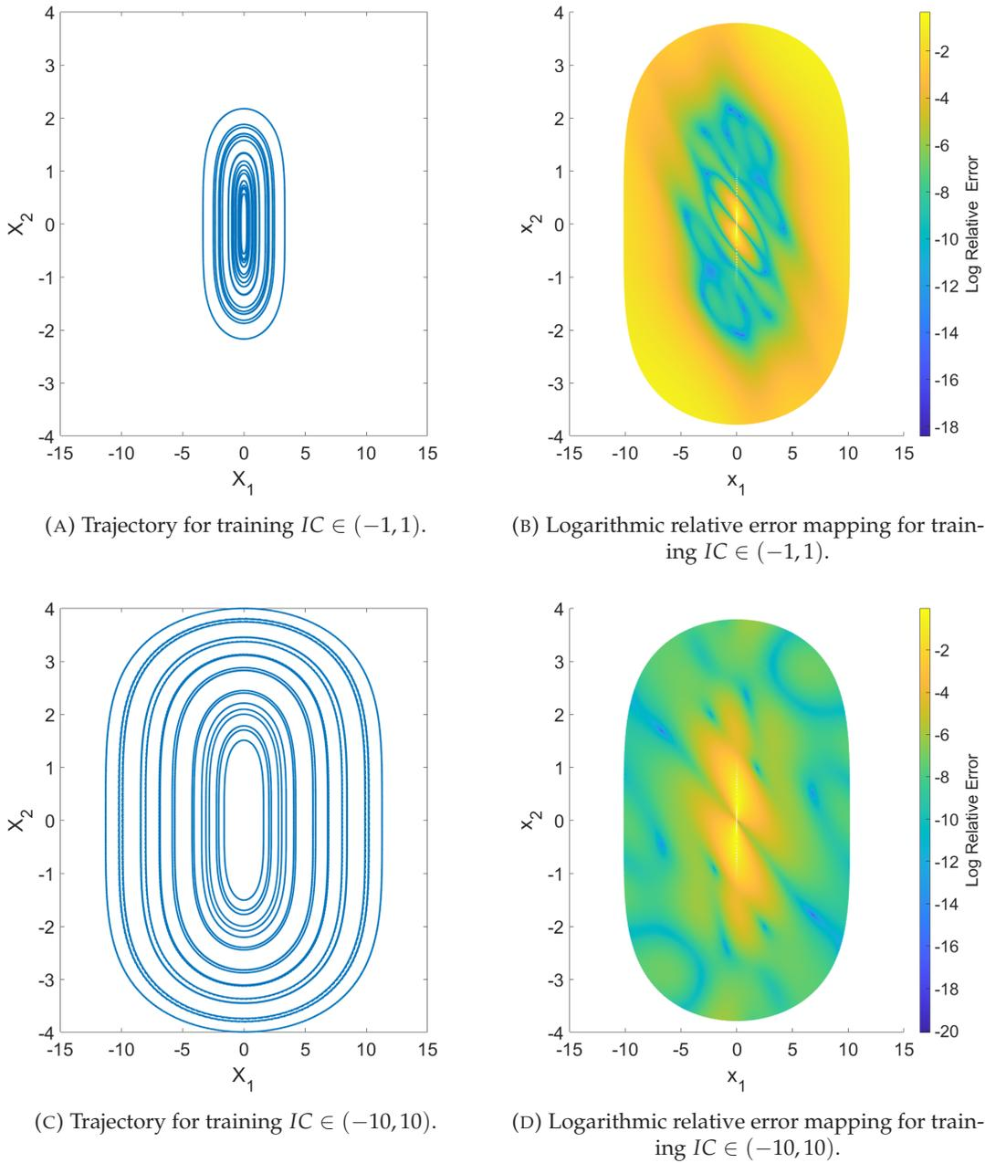
FIGURE 4.3: Impact of the size of the compact: Comparison of the autonomous system (Equation (4.20)) solutions for an observer defined in  $\mathbb{R}^3$ , with a different range for the Gaussian distributed initial conditions. The prediction test is over 100 equally distributed initial condition  $(x_{1,0}, x_{2,0}) \in [-10, 10]$ .
