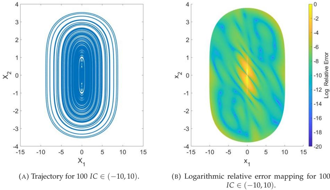
FIGURE 4.6: Solution for the autonomous system (Equation (4.20)) with an observer  $z$  defined in  $\mathbb{R}^3$ , with regular partition used for choosing the 100 initial conditions  $(x_{1,0}, x_{2,0}) \in (-10, 10)$ .
