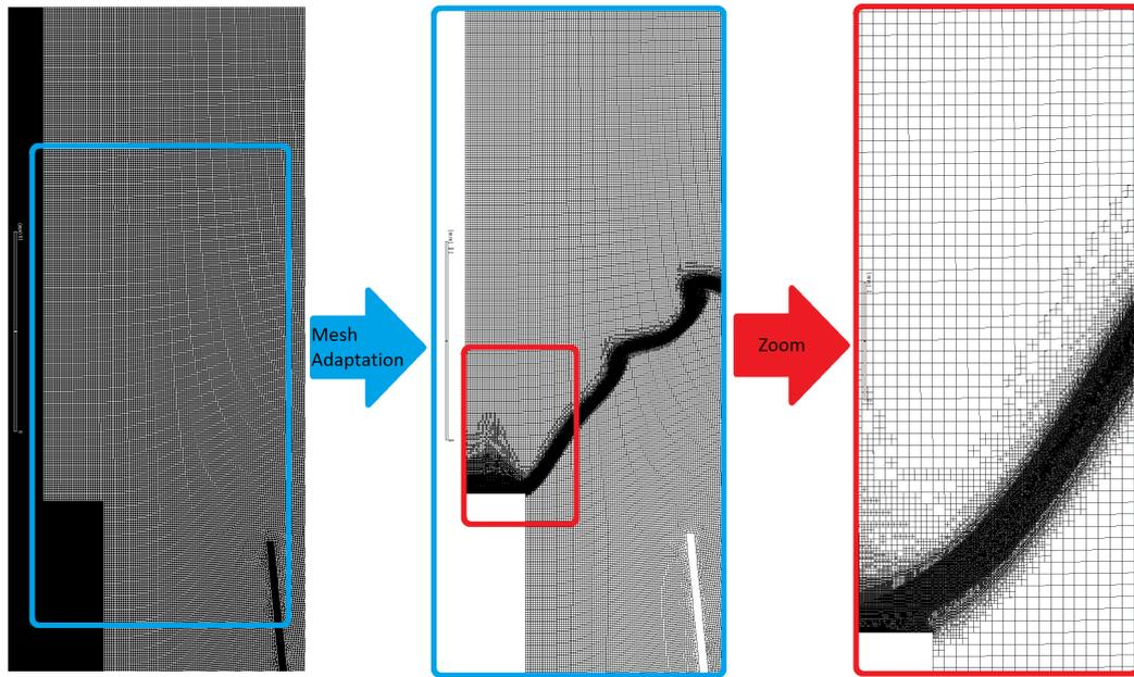
FIGURE 1.8: Representation of the mesh adaptation due to temperature gradient (obtained using Fluent). Left: base mesh with a size of  $100 \mu m$ ; center: mesh already adapted after the flame is developed; right: zoom on the adapted mesh.
