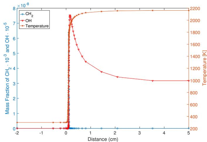
FIGURE 1.3: Fields of mass fraction of  $\text{CH}_2$  and  $\text{OH}$ , and temperature ( $K$ ) obtained for the 1D freely propagating laminar premixed methane/air flame, with equivalence ratio of  $\phi = 0.92$ ,  $T_\infty = 300\text{ K}$  and  $p = 1\text{ atm}$  [36].
