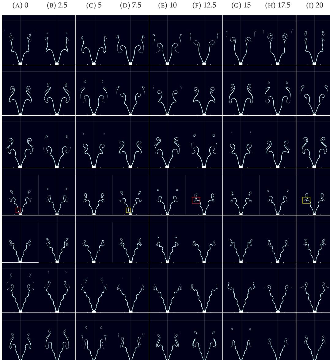
FIGURE 2.12: Flame front surface at different, equally spaced instants (by 2.5 ms), for different forcing frequencies. Each row presents a different forcing frequency, in the following order: 50, 75, 100, 125, 150, 172 and 200 Hz, corresponding to Strouhal numbers of 0.48, 0.71, 0.95, 1.19, 1.43, 1.63 and 1.9.
