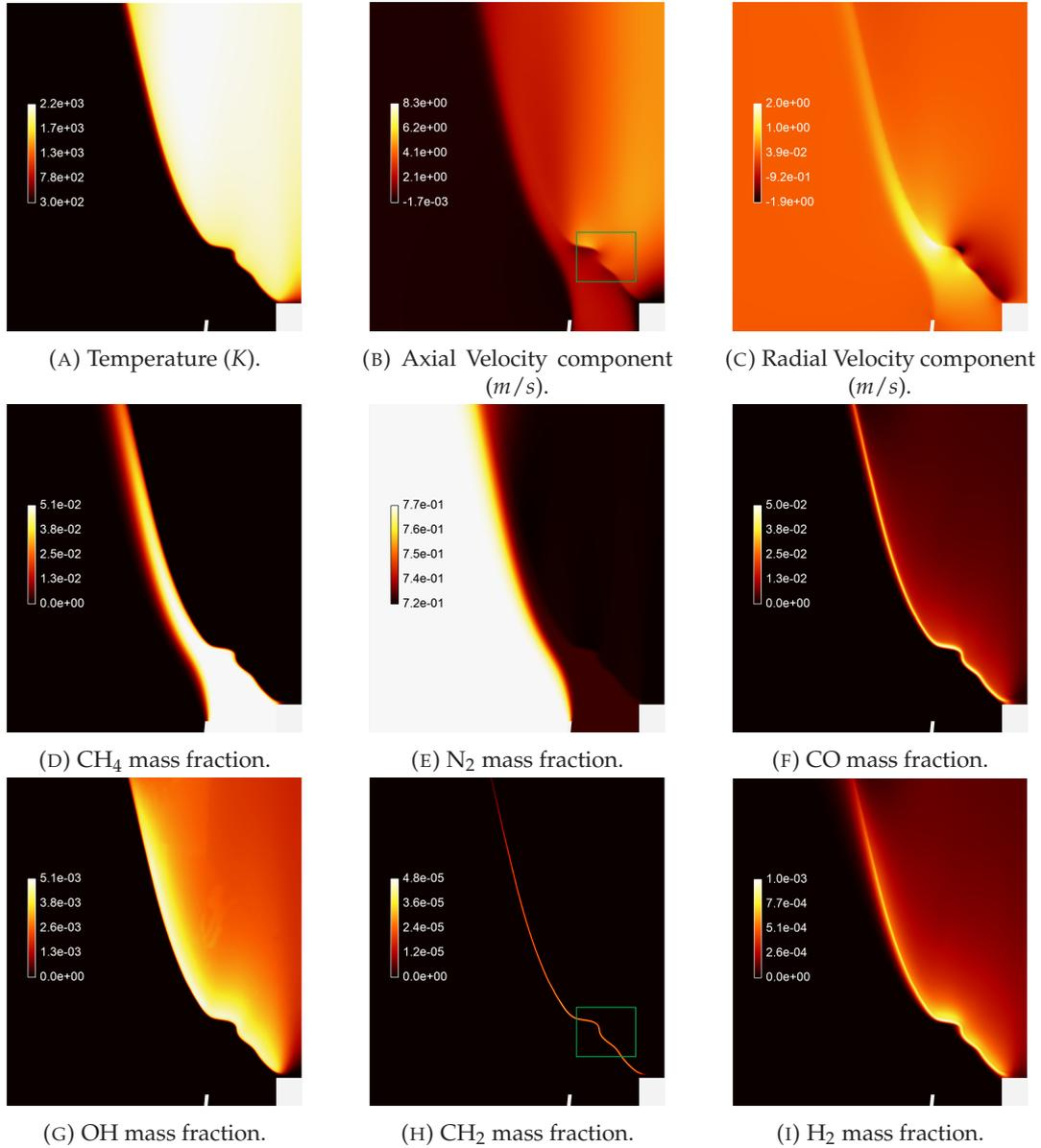
FIGURE 1.12: Structure of the laminar premixed inverted conical flame, with a volume flow rate of  $\dot{V}_d = 180.3 \text{ cm}^3/\text{s}$  and a methane/air equivalence ratio of  $\phi = 0.92$  [36].
