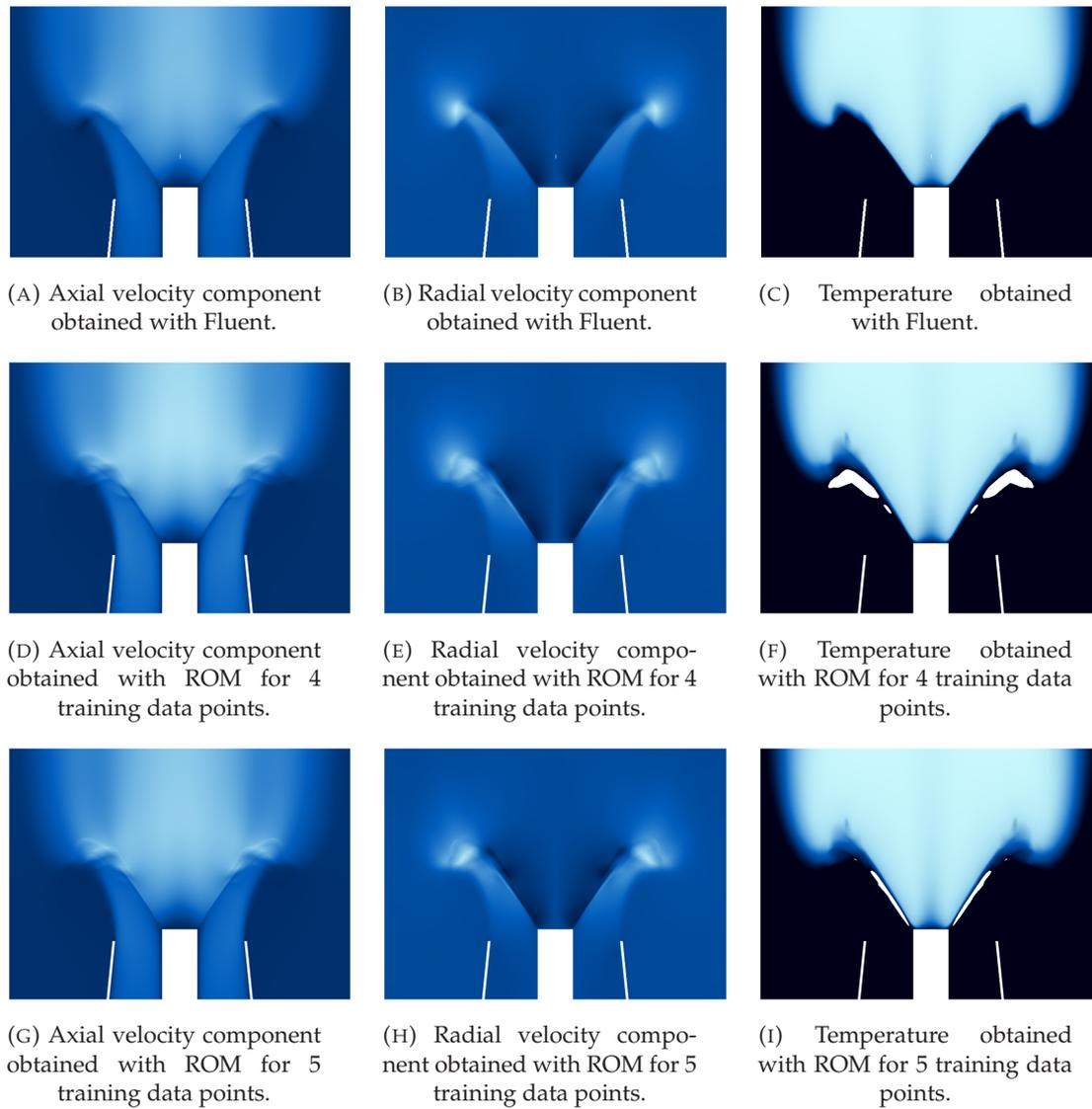
FIGURE 3.3: Comparison between the Fluent averaged results with ROM prediction for the averaged steady ICF, for a fuel inlet volume flow rate of  $\dot{V}_5 = 198.4 \text{ cm}^3/\text{s}$ . The colormap is defined as black an light blue at minimum values, respectively, i.e.,  $v_y \in [-1, 6] \text{ m/s}$ ,  $v_r \in [-2, 3] \text{ m/s}$  and  $T \in [298, 2200] \text{ K}$ .
