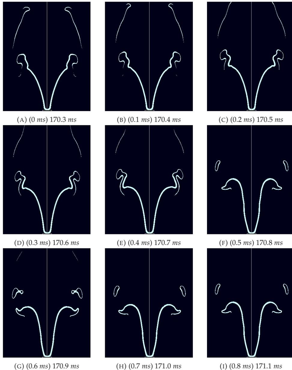
FIGURE 2.6: Unforced flame front position at different equally spaced (by  $100 \mu\text{s}$ ) instants in time.
