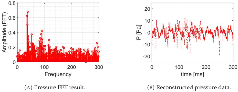
FIGURE 2.10: Unforced ICF pressure history frequency analysis and signal reconstruction. The depicted results are relative to the data extracted at point O (—), presented in Table 1.3.
