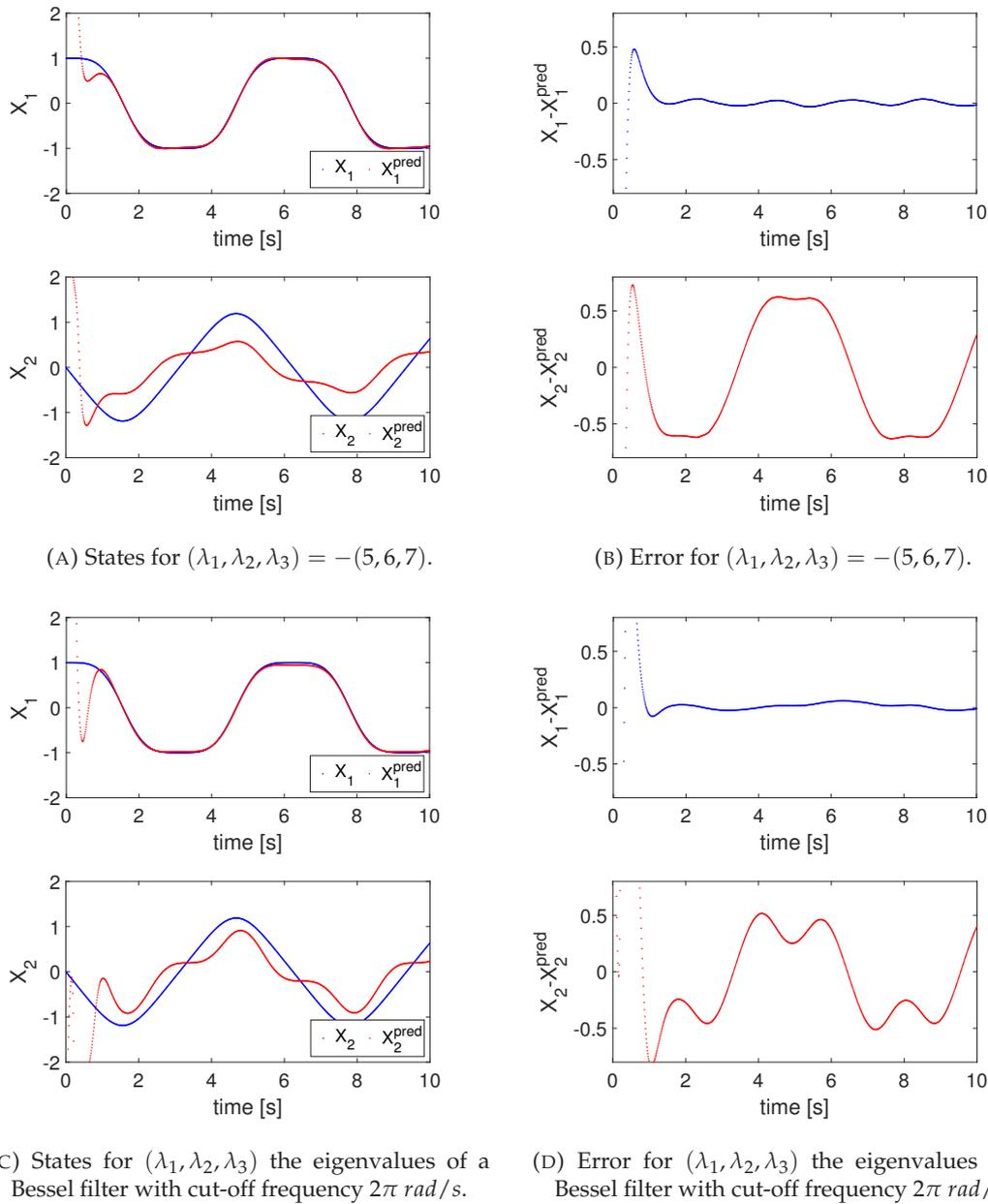
FIGURE 4.7: Evolution of the true and estimated states over time of the autonomous system (Equation (4.20)) for an observer defined in  $\mathbb{R}^3$ , with different eigenvalues.
