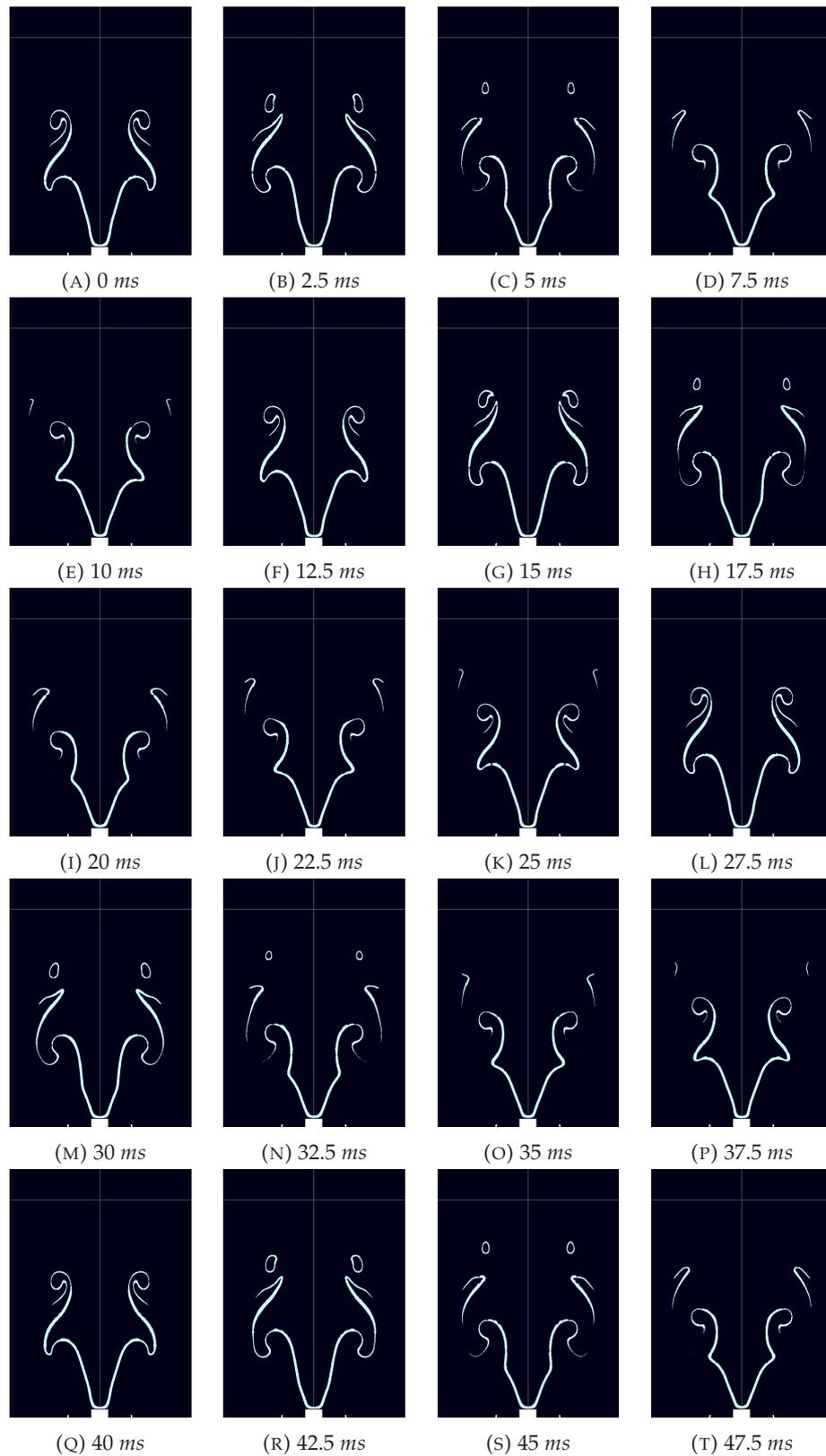
FIGURE A.2: Forcing of 75 Hz with adaptation 50 K/m.
