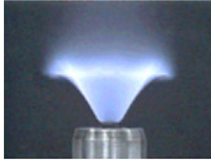
FIGURE 1.14: Experimental steady inverted conical flame, with equivalent ratio  $\phi = 0.92$  and nominal volume flow rate  $\dot{V}_d = 180 \text{ cm}^3/\text{s}$  [9].
