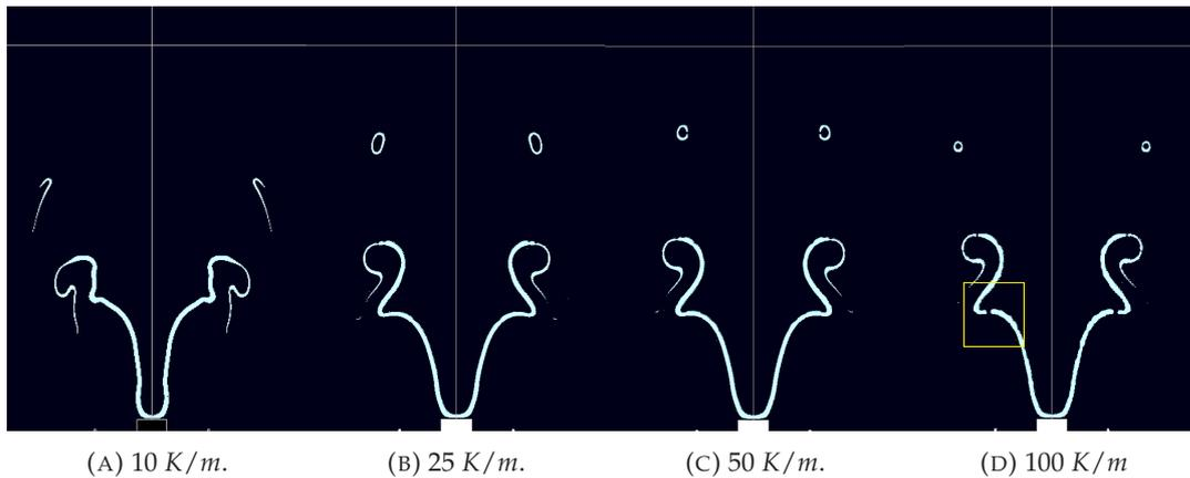
FIGURE 2.3: Instantaneous of the flame front for different mesh refinement temperature gradient threshold values.
