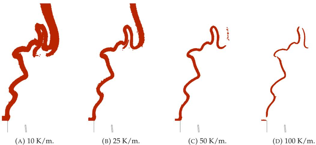
FIGURE 2.2: Mesh adaption region for different refinement temperature gradient threshold values.
