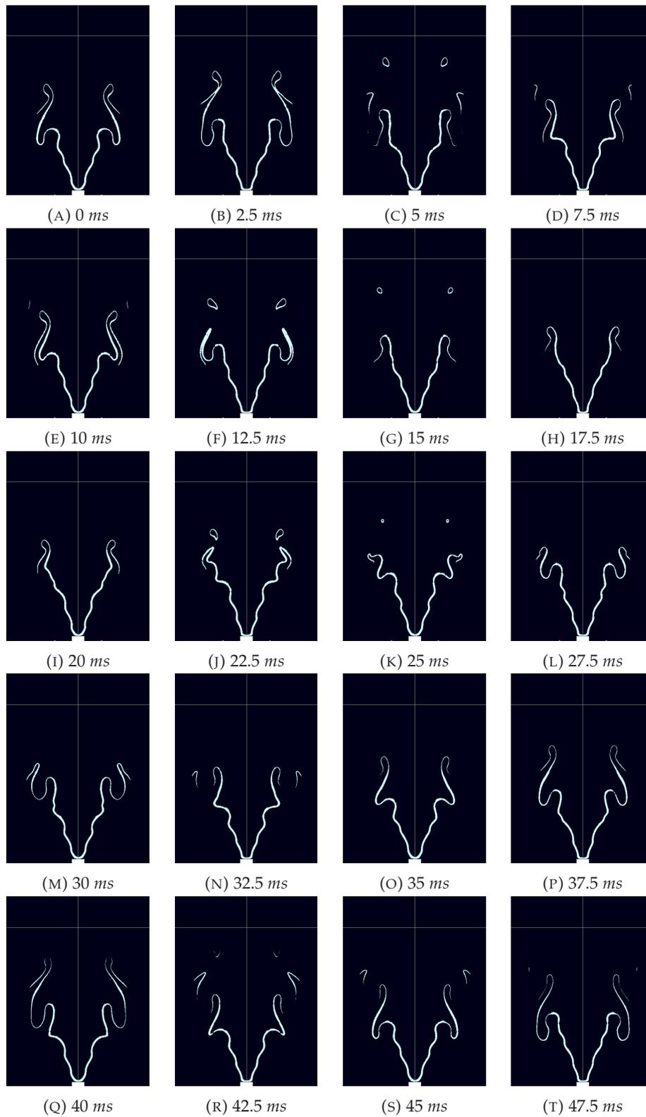
FIGURE A.7: Forcing of 200 Hz with adaptation 50 K/m.
