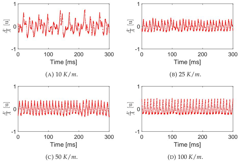
FIGURE 2.4: Flame surface area fluctuations results for each of the cases presented in Table 2.1, i.e., different mesh refinement thresholds.
