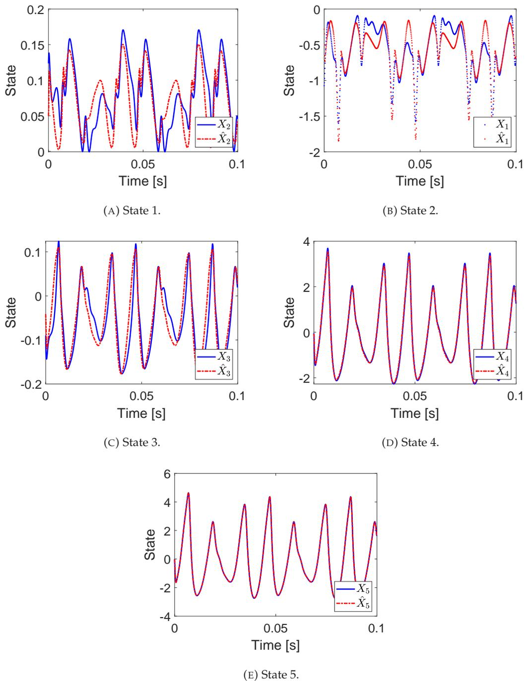
FIGURE 4.13: Comparison of the prediction for the trajectories with  $u(t) = 0.4 \cdot \sin(2\pi 100t) + 0.8 \cdot \sin(2\pi 150t)$ .
