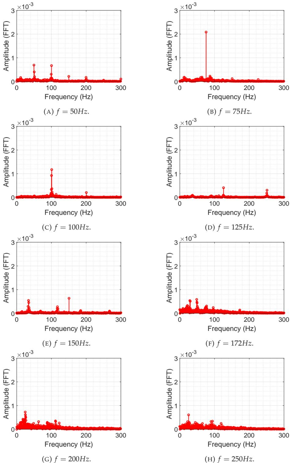
FIGURE 2.14: Harmonic response of the flame surface area fluctuation for different forcing frequencies ( $f$ ).
