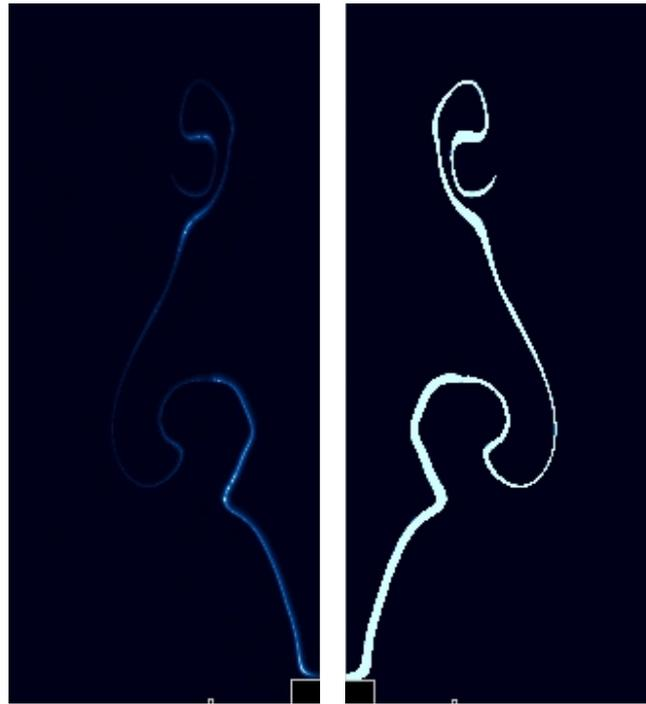
FIGURE 1.11: Comparison of the instantaneous flame front identified with the  $\text{CH}_2$  mass fraction (left) and with the binary field  $\iota$  (right).
