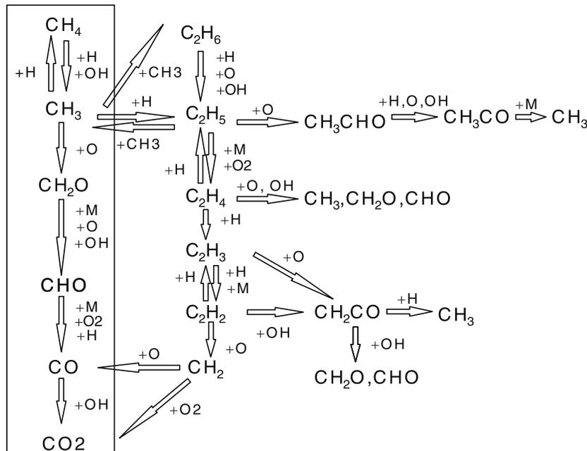
FIGURE 1.2: Simplified representative scheme of a detailed kinetic model for methane combustion [45].
