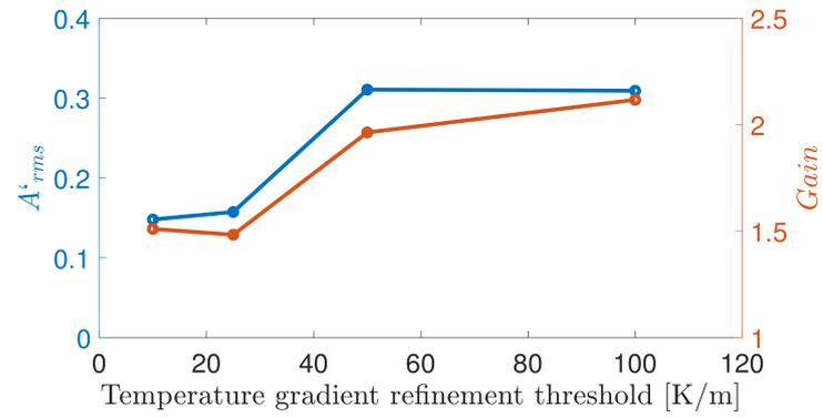
FIGURE B.1: RMS values of the flame surface area fluctuation [ $m^2$ ] and the corresponding FDF gain as a function of the temperature gradient refinement threshold.
