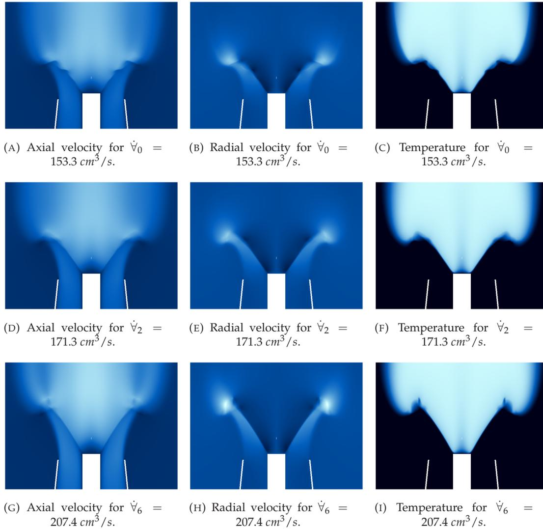
FIGURE 3.2: ICF training samples for the fields of velocity components and temperature, for three different fuel/air mixture flow rates. The colormap is defined as black to light blue at minimum values, respectively, i.e.,  $v_y \in [-1, 6] \text{ m/s}$ ,  $v_r \in [-2, 3] \text{ m/s}$  and  $T \in [298, 2200] \text{ K}$ .
