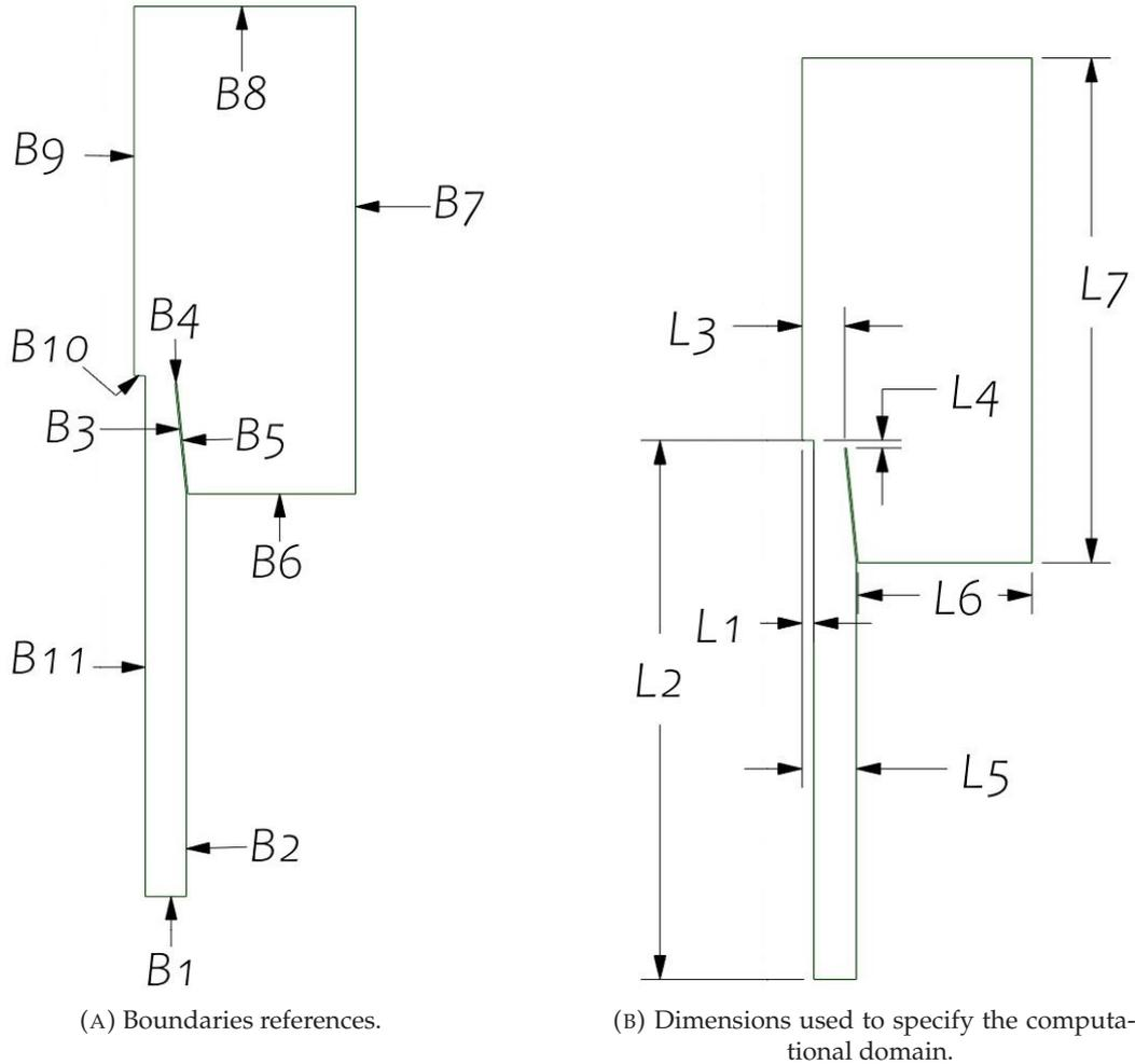
FIGURE 1.5: Representation of the axisymmetric computational domain with corresponding boundary conditions and dimensions labels. The boundary conditions setups and measures are given at Tabs. 1.1 and 1.2 respectively.
