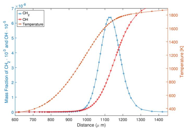
FIGURE 1.4: Zoom on the fields of mass fraction of  $\text{CH}_2$  and  $\text{OH}$ , and temperature ( $K$ ) obtained for the 1D freely propagating laminar premixed methane/air flame, with equivalence ratio of  $\phi = 0.92$ ,  $T_\infty = 300\text{ K}$  and  $p = 1\text{ atm}$  [36].
