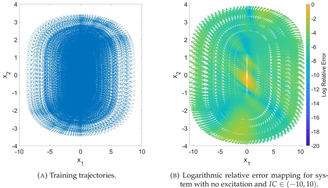
FIGURE 4.9: Training trajectories and estimation error for the artificially excited nonlinear oscillator.
