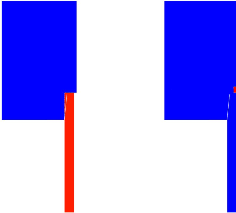
(A) Premixed fuel and air patch for the purpose of an isotherm computation. (B) Ignition patch for the purpose of a flame computation.
