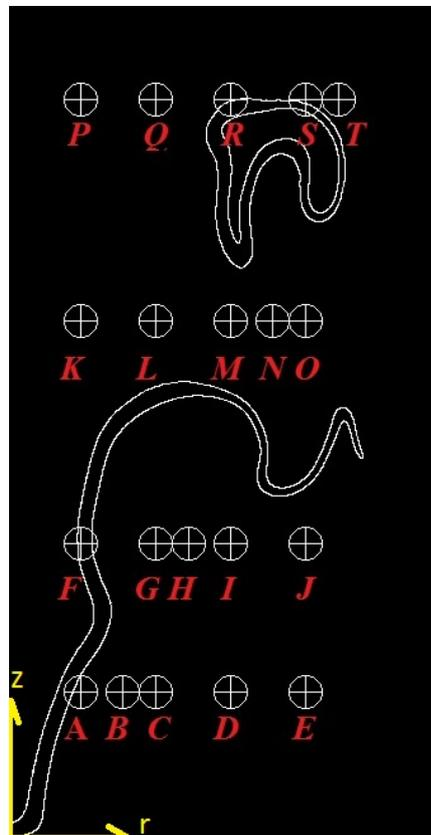
FIGURE 1.10: Data extraction points in the flame region and outline of fluctuation flame surface.
