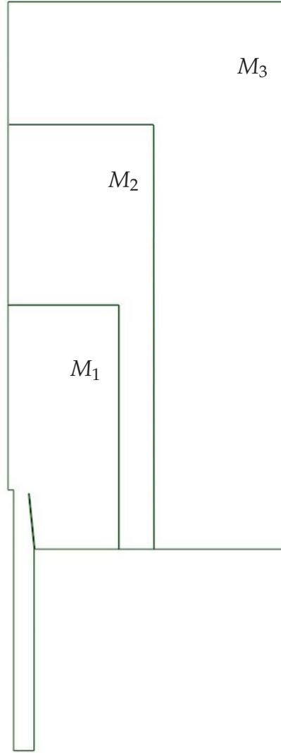
FIGURE 1.6: Axisymmetric computational domain blocks division.  $M_1$ : is the block where the flame is encountered;  $M_2, M_3$ : are the blocks where the air and burned gases flow.
