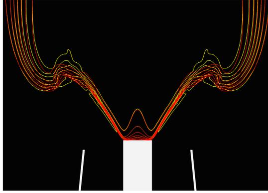
FIGURE 3.4: Comparison of the contour of the flame temperature for the ensemble averaged steady Fluent result (red) and the StaticROM prediction (yellow) for the ICF case 5, with a volume flow rate of  $\dot{V}_5 = 198.4 \text{ cm}^3/\text{s}$ . [36]
