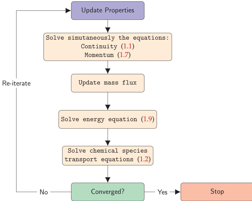
FIGURE 1.7: Flow chart representation for Fluent solution process.
