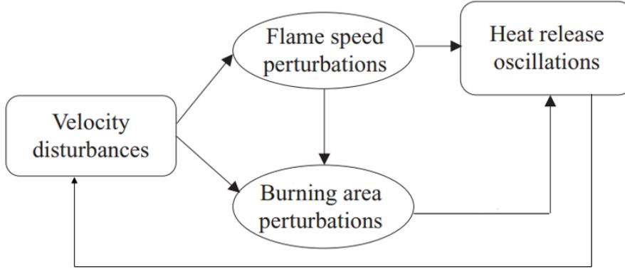
FIGURE 2.1: Resonant coupling mechanisms through which flow velocity oscillations lead to combustion heat release oscillations [71].
