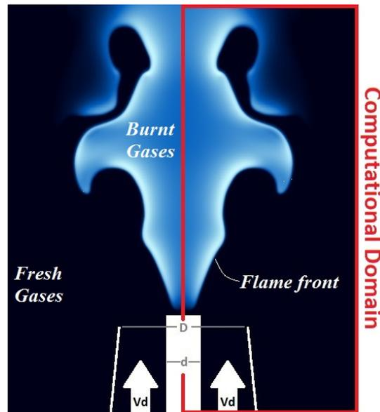
FIGURE 1.1: Representative view of OH mass fraction for the unsteady inverted conical flame. Mean velocity of  $v_d = 2.05 \text{ m/s}$  and methane/air equivalence ratio  $\phi = 0.92$ ,  $T_\infty = 300 \text{ K}$  and  $p = 1 \text{ atm}$  [36].
