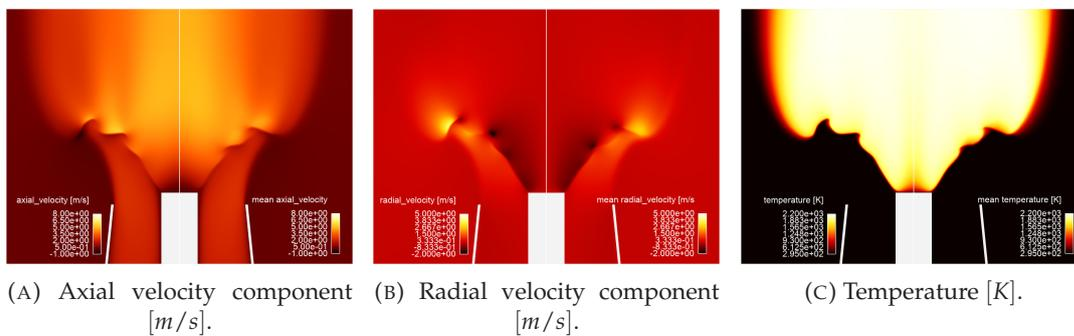
FIGURE 1.13: Comparison of the flame front structure between Fluent and its average: fields of velocity components and temperature, for two different fuel/air mixture flow rates. Fluent steady field on the left and ensemble average on the right side, for  $\dot{V}_3 = 180 \text{ cm}^3/\text{s}$ . [36]
