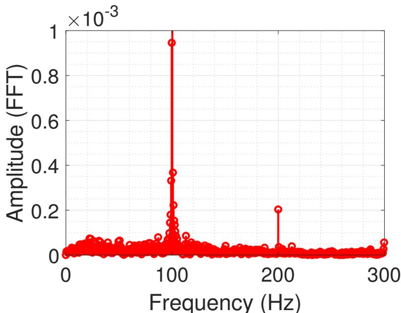
FIGURE 2.5: Spectrum of the heat release response for a mono-frequent excitation at  $f = 100$  Hz.
