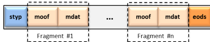
Figure 4.9 – Structure of a media segment with "eods" box.
