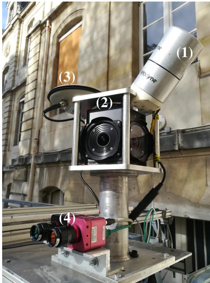
Figure 2.19: Sensors mounted on the roof of L3D2 vehicle: 1) Velodyne HDL-32E LiDAR; 2) Ladybug camera; 3) Antenna of GPS; 4) Hyperspectral cameras HS02 and HS03.
