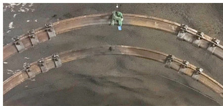
Figure 1.13: TH type steel ribs with sliding joints
