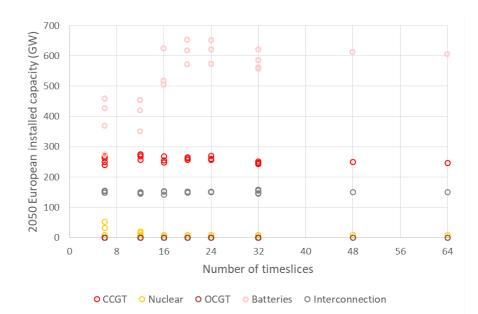
Figure A.7: Section 4.4.2: Impact of the number of timeslices on flexibility solutions 2050 European capacities in case B. Each dot corresponds to one of the variations of one of the 9 timeslice structures described in table 4.3.
