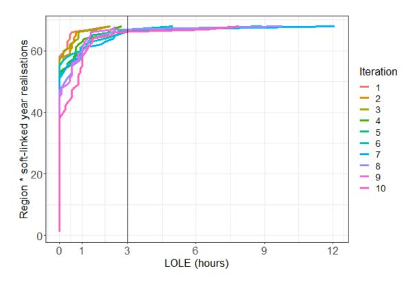
Figure 5.10: Evolution of LOLE over iterations for the "balanced" reserve margin update strategy, without capacity credit update. This graph should be read in the following way: out of the 68 LOLE values obtained in iteration 10 (one value for each of the 17 regions and each of the 4 soft-linked years), 47 were smaller or equal to 0.55 hours.
