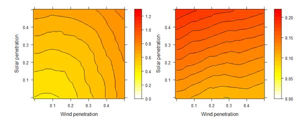
Figure 3.4: 95<sup>th</sup> percentile of annual flexible power requirement  $FPR_a$  in MW/MW (normalised by system maximum load, left) and energy requirement  $FER_a$  in TWh/TWh (normalised by system mean annual demand, right) in terms of wind and solar penetrations.
