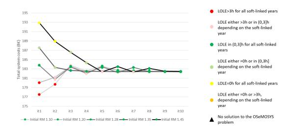
Figure 5.7: Evolution of OSeMOSYS total system costs over 10-iteration runs for the single-node German system, using the "balanced" reserve margin adjustment strategy, for different initial reserve margin (RM) sizes ranging from 1.10 to 1.45.
