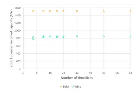
Figure A.4: Section 4.4.2: Impact of the number of timeslices on VRE 2050 European capacities in case A. Each dot corresponds to one of the variations of one of the 9 timeslice structures described in table 4.3.
