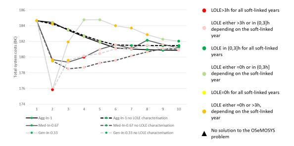
Figure 5.15: Evolution of OSeMOSYS total system costs over 10-iteration runs for the single-node German system, with (full lines) and without (dashed lines) LOLE characterisation. Flexibility proxies are based on the 80<sup>th</sup> percentile of FSCD.
