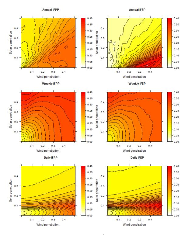
Figure A.2: Section 3.5.2: Based on the 95<sup>th</sup> percentiles of FPR and FER, interconnection flexible power potential (IFPP) expressed in terms of percentage of  $\sum_{c} FPR$  (left) and energy potential (IFEP) expressed in terms of percentage of  $\sum_{c} FER$  (right) in terms of wind and solar penetrations. Top, middle and bottom rows show results for the annual, weekly and daily timescales respectively.
