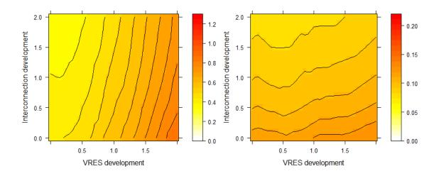
Figure 3.5: 95<sup>th</sup> percentile of normalised annual flexible power (left) and energy (right) requirement in terms of VRE and network developments.
