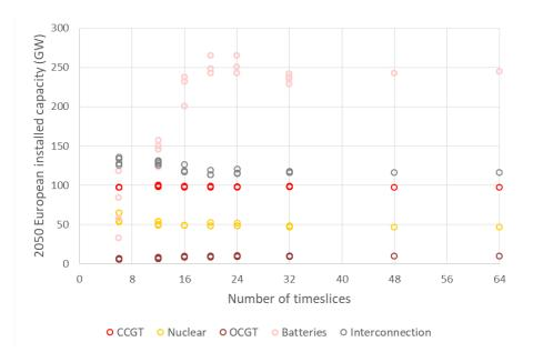
Figure A.5: Section 4.4.2: Impact of the number of timeslices on flexibility solutions 2050 European capacities in case A. Each dot corresponds to one of the variations of one of the 9 timeslice structures described in table 4.3.
