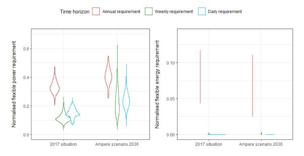
Figure 3.9: Flexibility requirements evaluated with I,  $p_{wind}$ ,  $p_{solar}$ ,  $p_{heat}$  and  $p_{cool}$  set at 2017 and Ampere scenario 2036 levels.
