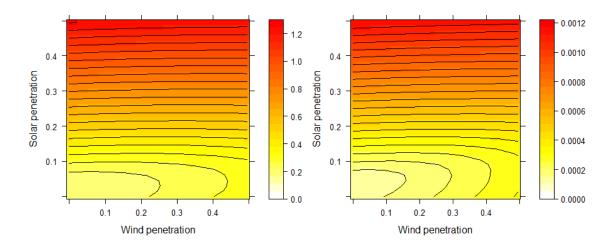
Figure 3.8: 95<sup>th</sup> percentile of normalised daily flexible power (left) and energy (right) requirement in terms of wind and solar penetrations.
