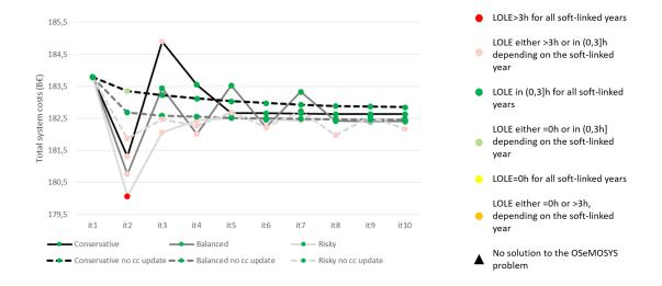
Figure 5.8: Evolution of OSeMOSYS total system costs over 10-iteration runs for the single-node German system, for different reserve margin adjustment functions with an initial reserve margin size of 1.28. Full lines show results for runs with capacity credit (cc) updates, dashed lines for runs without capacity credit updates.
