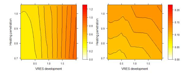
Figure 3.6: 95<sup>th</sup> percentile of normalised annual flexible power (left) and energy (right) requirement in terms of VRE and electric heating penetrations.
