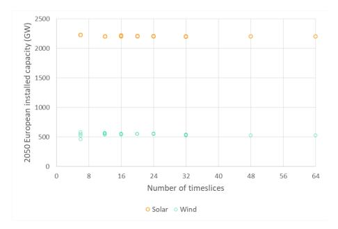
Figure A.6: Section 4.4.2: Impact of the number of timeslices on VRE 2050 European capacities in case B. Each dot corresponds to one of the variations of one of the 9 timeslice structures described in table 4.3.
