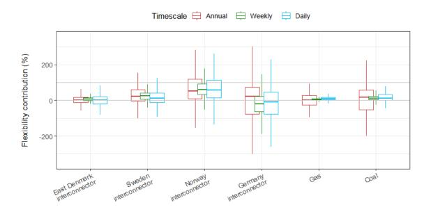
Figure 2.8: How do interconnectors contribute to flexibility in highly interconnected systems? Flexibility solution contribution distribution on annual, weekly and daily timescales, for the western Denmark power system in 2018 (data from [88]).
