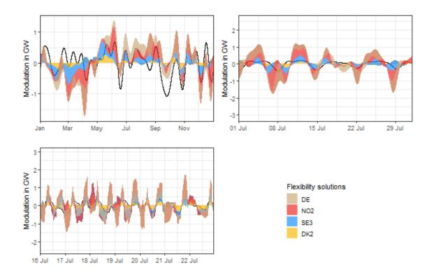
Figure A.1: Section 2.4.3: How do interconnectors contribute to flexibility in highly interconnected systems? Flexibility solution modulation stack on annual, weekly and daily timescales, for the western Denmark power system in 2018 (data from [88]). Note that the sum of the interconnector modulations do not sum up to total system modulation (black line), as, to ensure readability, other flexibility solution modulations have not been represented.
