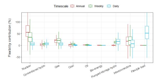
Figure 2.5: How do solutions currently contribute to flexibility? Flexibility solution contribution distributions on annual, weekly and daily timescales, on the French power system in 2018. Generation and interconnector flow data from [95], flexible load data was generated by an unpublished RTE model based on consumer panels.
