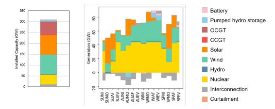
Figure 5.17: For the reserve margin feedback method applied to the 17 node case study, OSeMOSYS 2050 dispatch for the British Isles region over 16 timeslices. These results are those obtained for the cheapest adequate investment path proposed by the soft-linking framework ("balanced" reserve margin update, no capacity credit update, iteration 7). Note that while timeslice bars are given equal widths, they do not represent the same time duration (SUNI: summer night, AUMO: autumn morning etc.).
