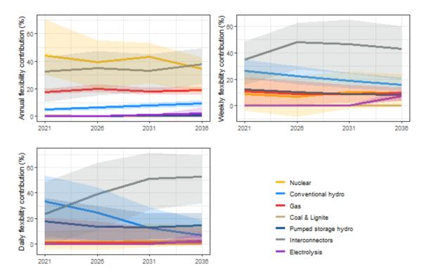
Figure 2.7: How could the roles of flexibility solutions evolve in the coming years? Evolution of flexibility solution contribution distribution between 2021 and 2036, on the French power system (data from the reference scenario used in [97, 98]). Uncertainty bounds correspond to the 25<sup>th</sup> and 75<sup>th</sup> percentiles of FSCDs, full lines correspond to the median.
