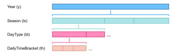
Figure 4.4: Hierarchical structure of OSeMOSYS timeslices. Lh specifies the number and order of the fractions of ld, ld those of the fractions of ls, and ls those of the fractions of lh.
