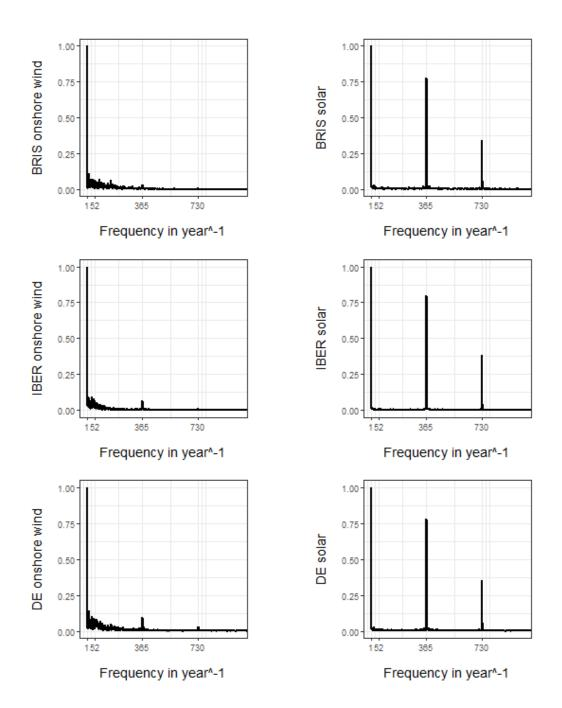
Figure A.3: Section 4.3.4: Normalised power spectral densities of onshore wind (left) and solar (right) hourly time series, for the British Isles (top row), Iberia (middle row) and Germany (bottom row). These were obtained based on 1 of the 35 weather years mentioned in section 4.3.4.
