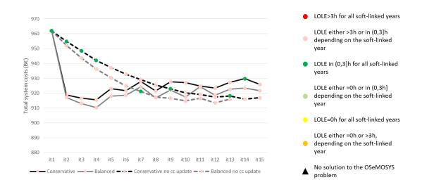
Figure 5.9: Evolution of OSeMOSYS total system costs over 10-iteration runs for the 17-node European system, for different reserve margin adjustment functions with an initial reserve margin size of 1.28. Full lines show results for runs with capacity credit (cc) updates, dashed lines for runs without capacity credit updates.
