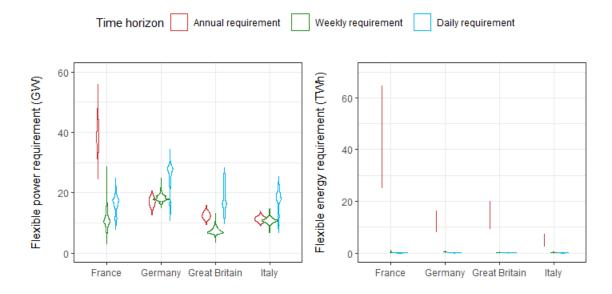
Figure 3.3: Flexibility requirements for different timescales and different countries. Electric heating and cooling levels are at 2017 levels, VRE generation has not been deducted from the load, interconnection has not been taken into account.
