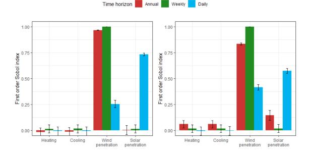
Figure 3.12: GSA results for interconnection flexible power (left) and flexible energy (right) potentials.
