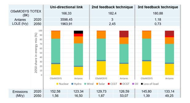
Figure 5.16: Comparison of a selection of OSeMOSYS and Antares outputs, for a uni-directional soft link and for the best adequate solutions proposed by the second and third feedback technique.
