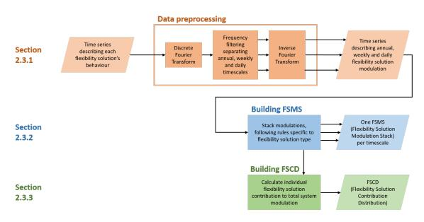
Figure 2.2: Overview of the methodology used to build FSMS and FSCD.
