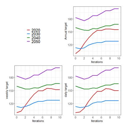
Figure A.11: Section 5.6.2: Evolution of flexibility target values for the model run of the single node German power system, an inertia set to 0.67 and flexibility targets adjusted using the "medium" strategy. Iterations 8 and 10 lead to LOLE levels under 3 hours. See Section 5.6.1 for information on how flexibility targets are defined and updated.
