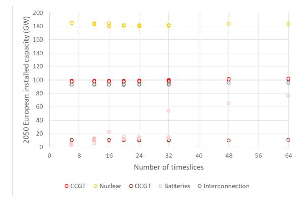
Figure 4.7: Impact of the number of timeslices on flexibility solutions 2050 European capacities. Each dot corresponds to one of the variations of one of the 9 timeslice structures described in Table 4.3.
