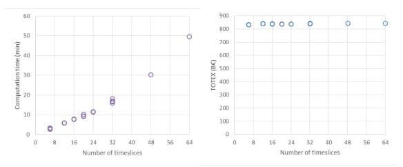
Figure 4.5: Impact of the number of timeslices on OSeMOSYS computation time (left) and TOTEX (right). Each dot corresponds to one of the variations of the 9 timeslice structures described in Table 4.3.
