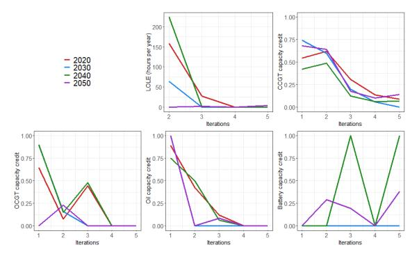
Figure 5.4: Evolution of loss-of-load-expectation and capacity credit values of CCGT, OCGT, oil power plants and batteries over iterations, for a reserve margin size of 0.75. Variations in capacity credit values suggest that they are not fulfilling their intended role: for dispatchable generation, the proportion of capacity that can be reliably expected to generate electricity during times of peak demand should be largely independent of system structure, and hence remain fairly constant.
