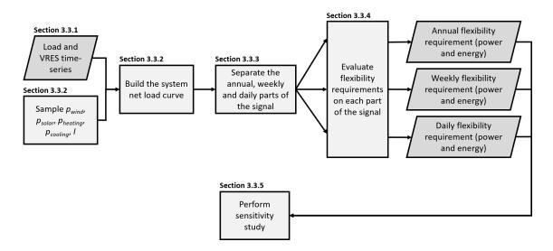
Figure 3.1: General overview of the proposed methodology. The process described in the top line is performed several tens of thousands of times, the resulting flexibility requirements are then fed the sensitivity study at the end of the chain.
