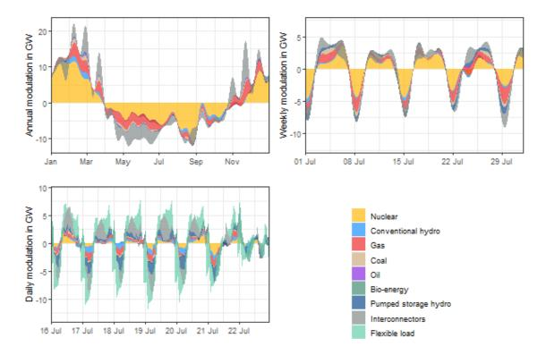
Figure 2.4: Who currently provides flexibility? Annual (top left), weekly (top right) and daily (bottom left) flexibility solution modulation stacks, on the French power system in 2018. Generation and interconnector flow data comes from [95], flexible load data was generated by an unpublished RTE model based on consumer panels.
