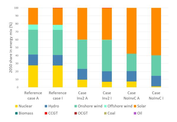
Figure 4.8: Annual contribution of considered generation technologies to total load, aggregated at the European level. For each case, the results are shown for the A and the I timeslice structures shown in Table 4.3.
