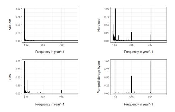
Figure 2.3: How different are the roles of flexibility solutions over different timescales? Normalised power spectral densities show the timescales over which behaviour is modulated, for nuclear, coal, gas and pumped hydro storage time series, on the German power system in 2018 (data from [88]). Marked out frequencies correspond to periods of a year, a week, a day and half a day.
