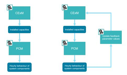
Figure 5.1: Relations between Capacity Expansion Models and Production Cost Models in a uni-directional (left) and bi-directional (right) soft-linking exercise.
