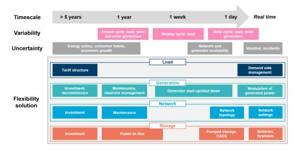
Figure 1.1: Different sources of variability and uncertainty generate a need for flexibility, which can be dealt with by a set of flexibility solutions. These are shown over a range of different timescales.
