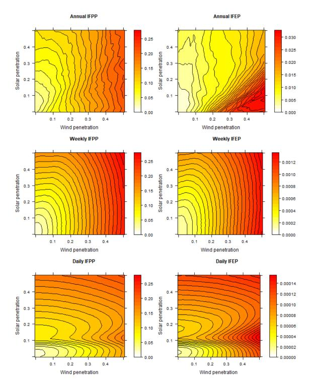
Figure 3.11: Based on the 95<sup>th</sup> percentiles of FPR and FER, interconnection flexible power potential (IFPP) in GW (left) and energy potential (IFEP) in TWh (right) in terms of wind and solar penetrations. Top, middle and bottom rows show results for the annual, weekly and daily timescales respectively.
