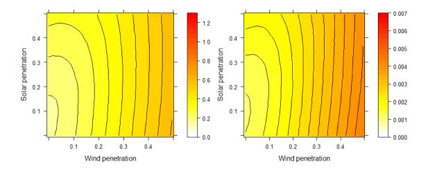
Figure 3.7: 95<sup>th</sup> percentile of normalised weekly flexible power (left) and energy (right) requirement in terms of wind and solar penetrations.
