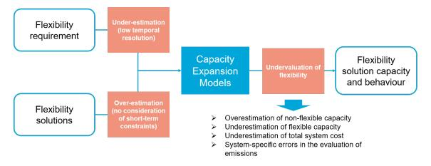
Figure 4.1: Simplifications made in Capacity Expansion Models cause flexibility to be undervalued. This leads to errors in optimal installed capacities, total system cost and emissions.
