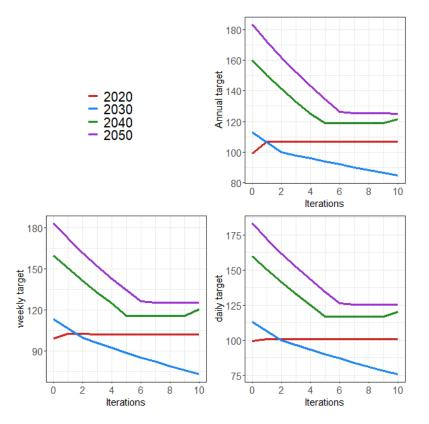
Figure A.10: Section 5.6.2: Evolution of flexibility proxy values for the model run of the single node German power system, an inertia set to 1 and flexibility targets adjusted using the "aggressive" strategy. Iterations 2 through 9 lead to LOLE levels under 3 hours.
