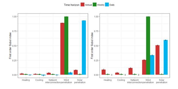
Figure 3.10: GSA results for flexible power (left) and flexible energy (right) requirements.
