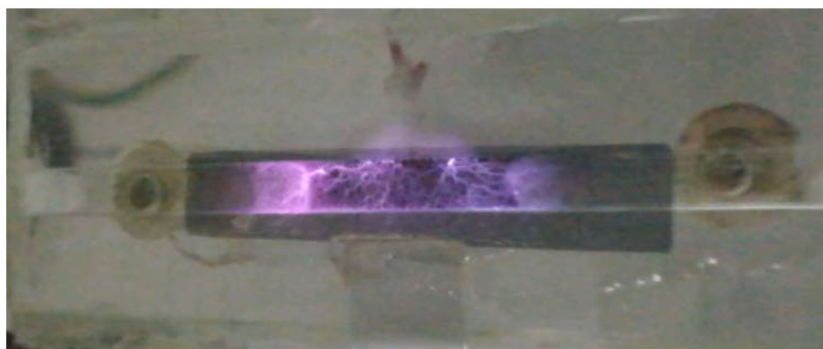
Figure 5-2. DBD plasma created in milli-reactor with ITO as electrode (Argon, applied voltage = 8.0 kV, f = 42 kHz, reactor configuration (Figure 5-1a))
