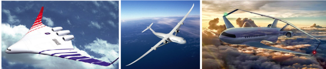
Figure 1.1: Possible architectures for the civil transport aircraft of the future: Blended Wing Body (BWB) , Truss Braced Wings (TBW) and PrandtlPlane (PrP) concepts
