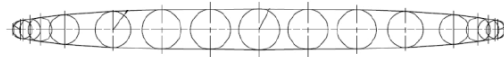
Figure 4.22: Example of bidirectional sections for application to air-cooling systems, Spasic et al. [2012]
