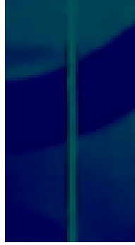
Figure 38: Oil injection at 17 °C in air at atmospheric pressure under an injection pressure of 30 bars through the 150 μm orifice diameter atomizer.
