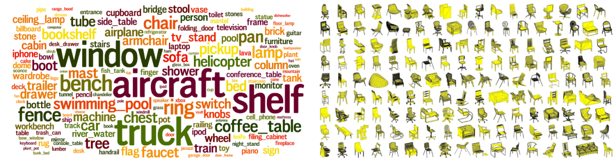
Figure 2.12 Left: word cloud visualization of the ModelNet dataset based on the number of 3D models in each category. Larger font size indicates more instances in the category. Right: Examples of 3D chair models. Image Source Zhirong Wu et al. (2015) .
