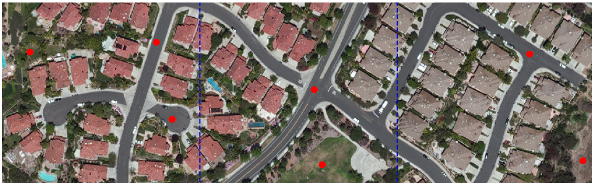
Figure 4.8 Image used to validate streaming version of the segmentation methods. The image has been split in three blocks (see blue dashed lines) and the blocks stream from left to right. As explained in Section 4.2 two consecutive blocks share a column of pixels. In red, the pixels used as markers for watershed-cut.
