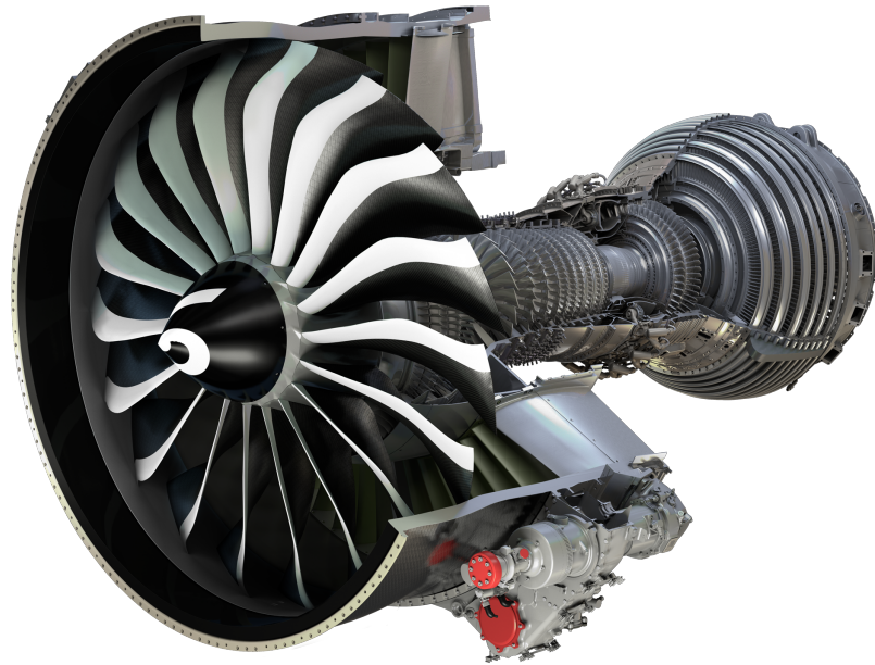
Figure 1.1: The LEAP, turbofan developed by CFM International, a joint venture between Safran Aircraft Engines and GE Aviation. This engine powers Airbus A320neo, Boeing 737 MAX and COMAC C919 planes. Picture taken from https://medialibrary.safran-group.com/Photos/media/178745 . ©2017 Antonio Gomez, Safran.
