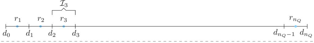
Figure 4.2 – Quantization model: interval limits and reconstruction values.
