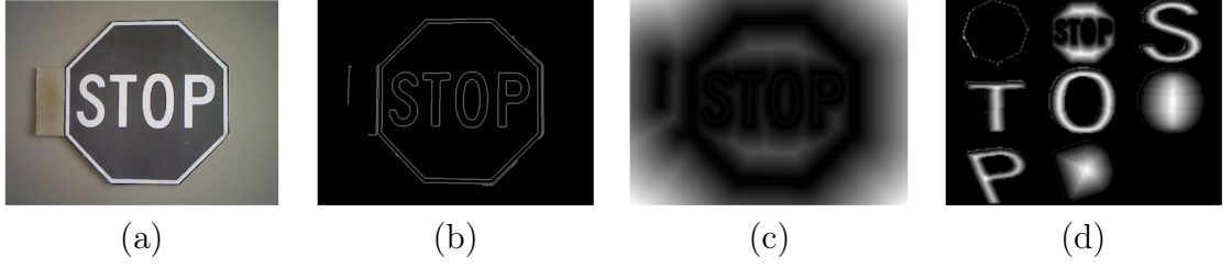
Figure 2.1: Figure from (Holzer et al., 2009). Given an input image (a), the corresponding edge image is obtained by applying a Canny detector (b), the distance transformation is computed from the edge image (c) and a set of templates are extracted for comparison (d).
