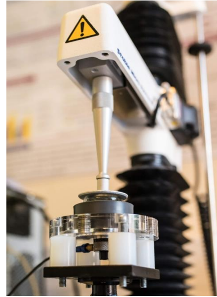
Figure 2.24: Uniaxial compression set up with PVC based tongue mimic.
