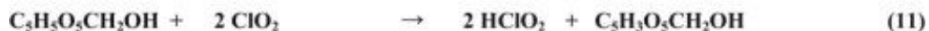
Fig. 2. Main reactions involved in the quenching process for chlorine, monochloramine and chlorine dioxide.
