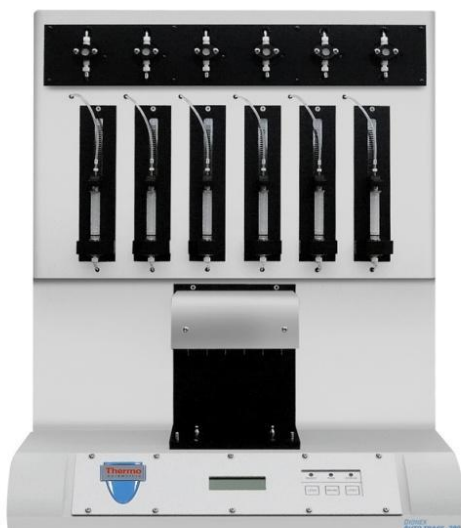
Figure II-1. Automate SPE Autotrace 280 (Thermo Fisher Scientific, Courtaboeuf, France)
