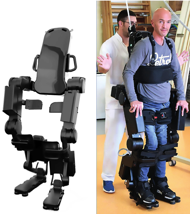
Figure 1.3: The exoskeleton Atalante ( https://www.wandercraft.eu/ ), walking with a paraplegic patient in a rehabilitation center .
