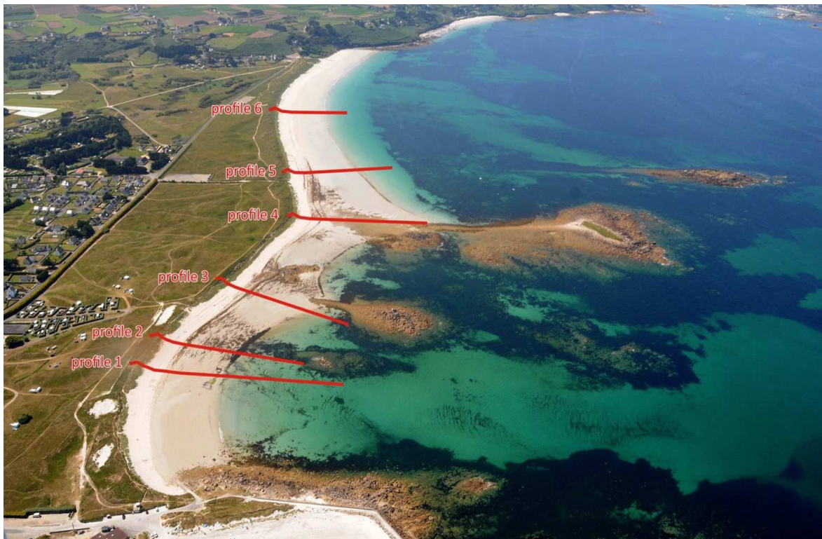
Figure II.2: Vougot Beach aerial view: Vougot Beach aerial photography seen from the eastern extremity, with the addition of the location of the 6 cross-shore profiles (named PF1, PF2, PF3, PF4, PF5, and PF6). crédit: Serge Suanez and géosAEL
