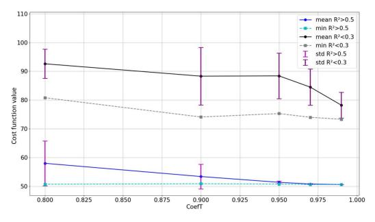
Figure III.4: Effect of changing CoefT on the cost function value for 10 realizations of the model optimisation at profile 6 for a well-reproduced contour position time series ( $\mathbb{R}^2 > 0.5$ ) showing the mean value, the standard deviation and the minimum value of the cost function and on a badly reproduced contour position time series ( $\mathbb{R}^2 < 0.3$ )
