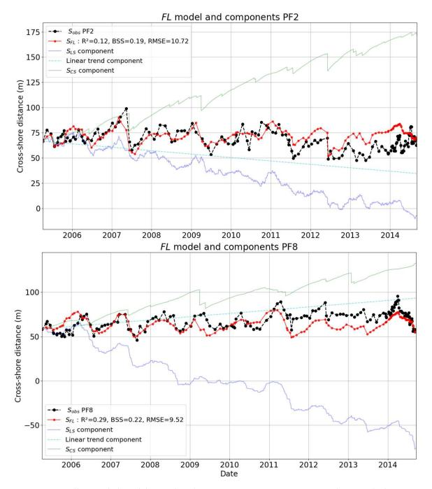
Figure V.17: Fully coupled model, FL shoreline position time series at PF2 and PF8 with the cross-shore  $S_{CS}$ , longshore  $S_{LS}$  and linear trend term component contribution.
