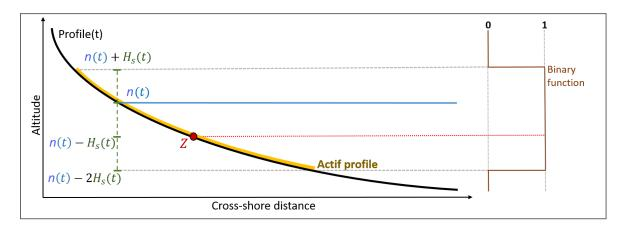
Figure III.2: Scheme of the adaptation of Lemos et al. (2018) of the equilibrium model to account for water level  $\eta$  depending on a threshold based on the wave height  $H_s$
