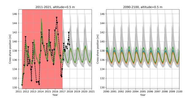
Figure VI.7: Empirical cross-shore model application at profile 6 of Vougot Beach at MSL (z=0.5m), using the projected wave time series from different RCP scenarios generate following the approach of Banno & Kuriyama (2014) (same color legend as Fig. VI.6): zooms of (a) the first 10 years (showing the calibration period in the shaded red zone) and (b) the last 10 years of the simulation period.
