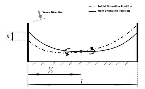
Figure I.11: Conceptual schematic of shoreline rotation on pocket beach, from (Turki et al. 2013).
