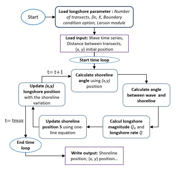
Figure IV.1: One-line longshore model conceptual functioning
