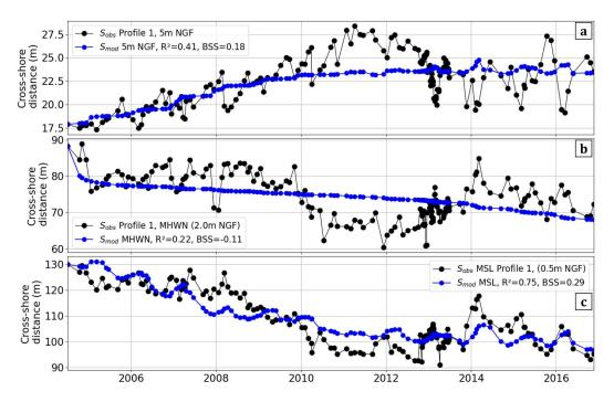
Figure III.8: Modeled contour position  $S_{mod}$  (blue), versus observations  $S_{obs}$  (black) for profile 1 at three elevations: (a) Upper Beach (Z=5 m NGF), (b)  $\approx$  Mean High Water Neap (Z=2.0 m NGF), and (c) Mean Sea Level (Z=0.5 m NGF).
