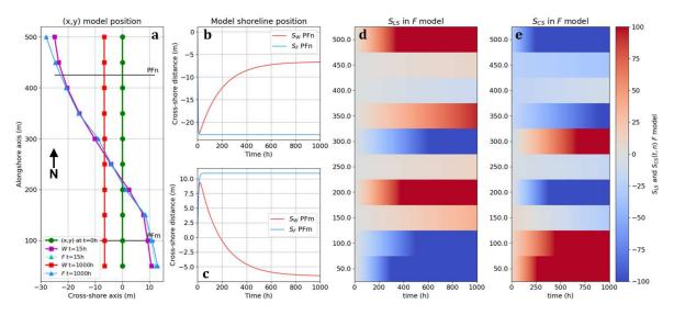
Figure V.4: Synthetic test case to illustrate the difference between the weakly coupled W and the fully coupled F models: (a) model x, y position at t=0, t=15h and t=1000. (b-c) Model shoreline positions  $S_W$  (red) and  $S_F$  (light blue) at 2 locations, (d) longshore model shoreline position  $S_{LS}$  in the F model, and (e) cross-shore model shoreline position  $S_{CS}$  in the F model as a function of time at each transect position.
