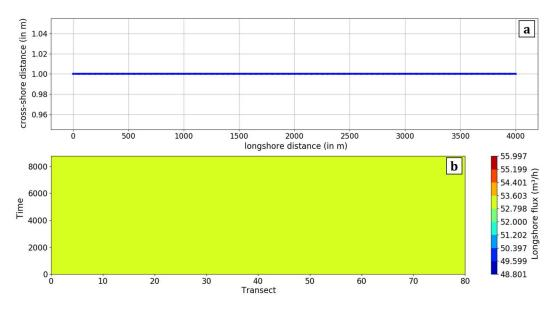
Figure IV.4: No flux test case: (a) Shoreline position evolution, (b) longshore sediment flux Q in time and space showing a constant and uniform flux value.
