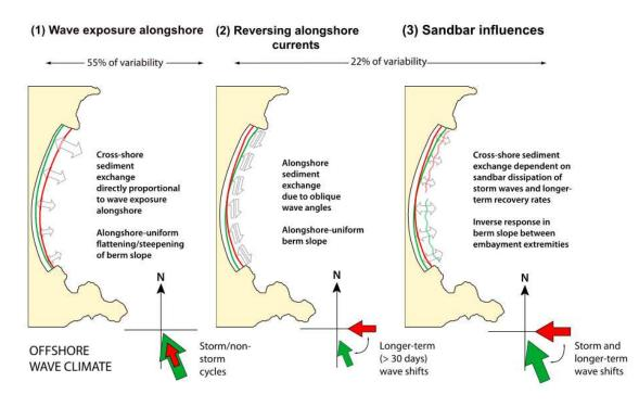
Figure II.6: Conceptual model of the 3 different planform rotation modes observed in (Harley et al. 2015). The red/green arrows represent the direction and magnitude of the offshore wave climate associated with the respective red/green embayed beach planform, while the grey arrows represent the magnitude and direction of sediment transport (scheme from Harley et al. (2015))
