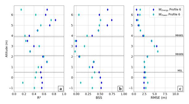
Figure III.15: Model statistics for profile 6 at Vougot Beach as a function of the elevation along the intertidal profile when using wave energy or wave power as the forcing wave condition: (a)  $R^2$ , (b) Brier Skill Score (*BSS*), and (c) *RMSE*.
