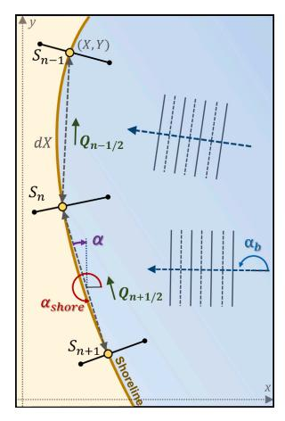
**Fig. 3.** Schematic representation of the model setup for cross-shore transects (index *n*), showing the shoreline position *S*, the relative wave angle  $\alpha$  (Eq. (4)), the alongshore sediment flux *Q*, and the local reference frame (*x*, *y*).
