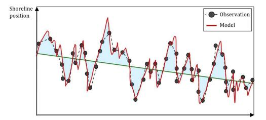
Figure V.7: Medium term criterion conceptual scheme representing the *BSS* calculation with the observations, the model, and the linear regression of the model (the baseline). The blue area corresponds to the model improvement compared to the baseline, assumed here mainly to account for the reproduced seasonal and intra-annual scales.
