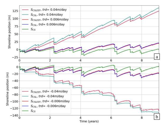
Figure V.1: Comparison of the linear term integration effects on model behavior for 2 different amplitudes of (a) positive linear trend, (b) negative linear trend. With  $S_{CSL}$ : model version with sum of the 2 independent components, and  $S_{CSLEEF}$ : model with the integration of the linear term in the equilibrium equation.
