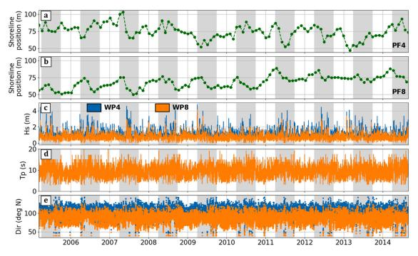
**Fig. 2.** Observations of the shoreline position (z=0 m altitude) at (a) PF4 and (b) PF8, and the corresponding wave conditions at WP4 (blue) and WP8 (orange) showing the: (c) significant wave height ( $H_s$ ), (d) peak wave period ( $T_p$ ), and (e) wave direction. The gray-shaded areas indicate austral winters. (For interpretation of the references to color in this figure legend, the reader is referred to the web version of this article.)
