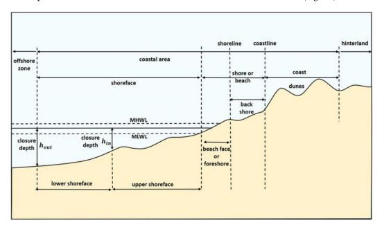
A beach profile can be divided in different areas based on the water level (Fig. I.4).
