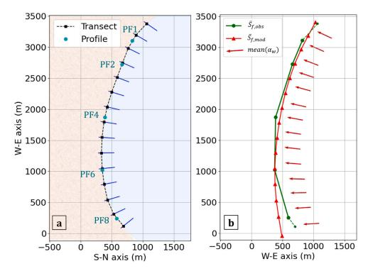
**Fig. 4.** (a) Longshore model setup at Narrabeen beach, showing the 15 defined cross-shore transects. (b) Observed (green line) and simulated (red line) annual mean shoreline position at the end of the 10-year simulation. For each cross-shore transect, the red arrow indicates the temporal mean wave angle ( $\alpha_w$ ) at 10 m water depth. (For interpretation of the references to color in this figure legend, the reader is referred to the web version of this article.)
