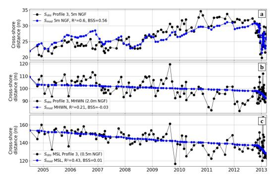
Figure III.9: Model contour position  $S_{mod}$  (blue), versus observation  $S_{obs}$  (black) for profile 3 at three elevations: (a) Upper Beach altitude (5 m NGF), (b)  $\approx$  Mean High Water Neap altitude (2.0 m NGF), and (c) Mean Sea Level (0.5 m NGF).
