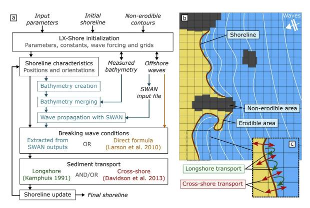
Figure I.13: LX-Shore model showing the (a) global framework and (b) cellular conceptual scheme, from (Robinet et al. 2020).
