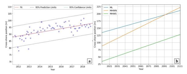
Figure VI.5: Linear extrapolation method applied to profile 6 at Vougot Beach: (a) Example calculated linear regression (in red) of the shoreline position observations (blue points) at MHWN elevation. (b) Linear extrapolation of the shoreline position at MSL, MHWN and MHWS elevations from the present to the year 2100 (figure from Cailler (2019)).
