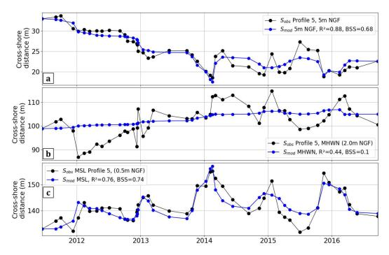
Figure III.10: Model contour position  $S_{mod}$  (blue), versus observation  $S_{obs}$  (black) for profile 5 at three elevations: (a) Upper Beach altitude (Z=5 m NGF), (b)  $\approx$  Mean High Water Neap altitude (z=2.0 m NGF), and (c) Mean Sea Level (z=0.5 m NGF).
