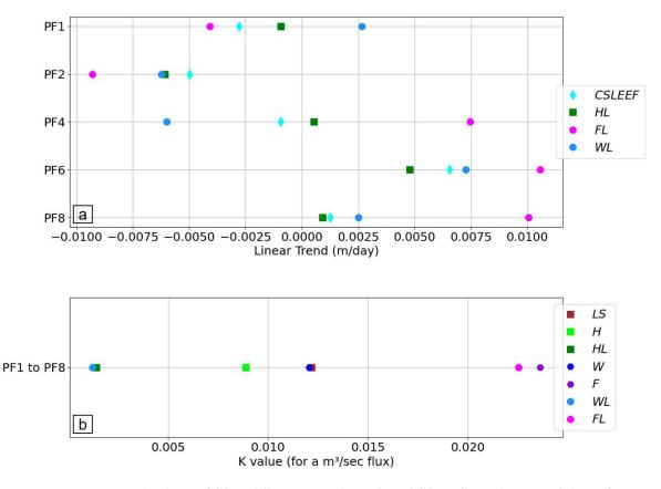
Figure V.9: Optimized values of (a) trd (linear trend term) and (b) K (longshore model coefficient, constant for all profiles) at Narrabeen Beach for each model formulation.
