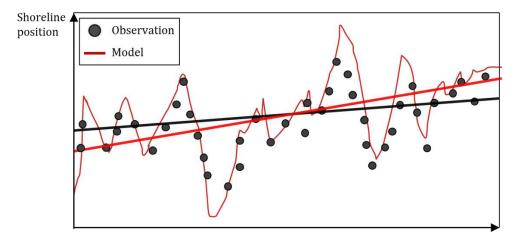
Figure V.8: Long term criterion conceptual scheme representing the observations, the model shoreline position, and their respective linear regressions in black and red, highlighting the difference in slope between the 2 regressions used as criteria.
