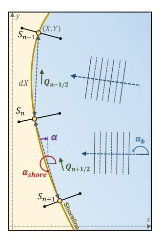
Figure IV.2: Schematic representation of the model setup for three cross-shore transects (index n), showing the shoreline position S, the relative wave angle  $\alpha$  (eq. IV.4), the alongshore sediment flux Q, and the local reference frame (X, Y).
