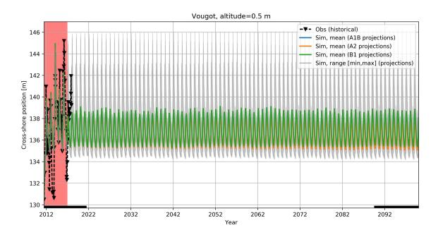
Figure VI.6: Empirical cross-shore model application at Profile 6 of Vougot Beach at MSL (z=0.5m) from 2011 to 2100, using the projected wave time series from different RCP scenarios generated following the approach of Banno & Kuriyama (2014). The shaded red zone indicates the model calibration period.
