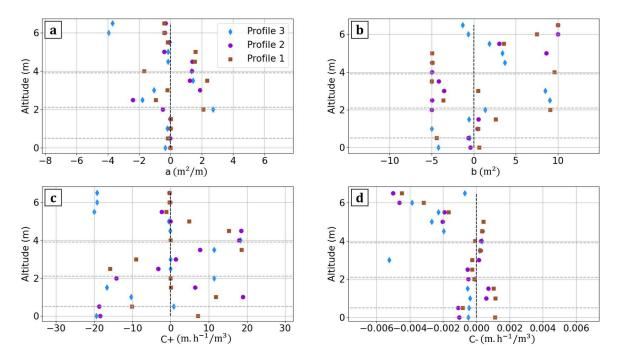
Figure III.11: Optimized model coefficients as a function of altitude for profile 1 (brown), 2 (purple), and 3 (light blue) for (a) coefficient a, (b) coefficient b, (c) coefficient  $C^+$ , (d) coefficient  $C^-$ .
