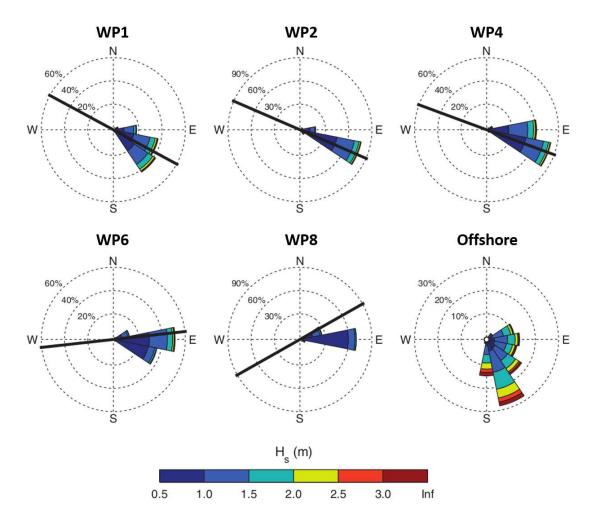
Figure II.5: Wave roses in 10 m water depth offshore of each profile and in 80 m water depth 11km offshore at the Sydney wave buoy. The black line indicates the respective profile transect orientation (from Turner et al. (2016)).
