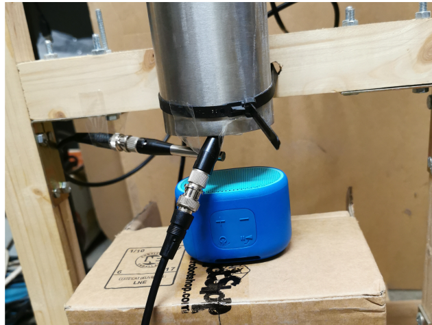
Figure ii.15: Acoustic parameter identification setup.
