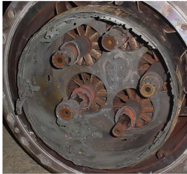
Figure 1.2: Burner assembly that has been damaged by thermoacoustic instabilities. From [Goy et al. 2005].
