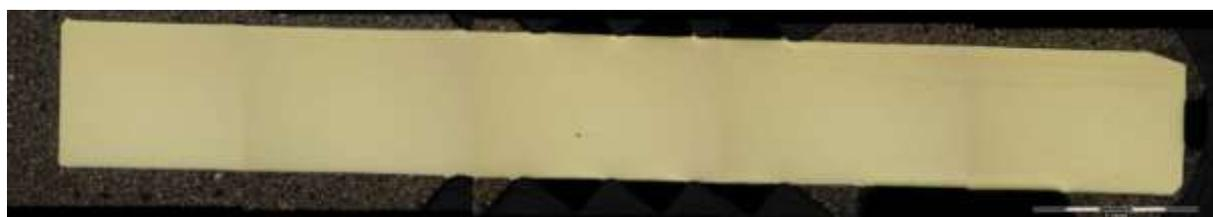
FIGURE 96: PASTILLE FRITTEE AVEC LE CYCLE DE REFERENCE AVEC POST TRAITEMENT
