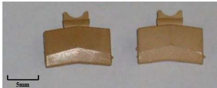
FIGURE 37 : COMPARAISON DES PIÈCES INJECTÉE (A GAUCHE) ET DELIANTÉE (A DROITE) EN OR 18 CARATS JAUNE
