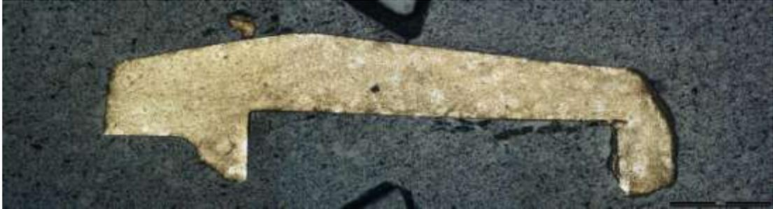
FIGURE 63 : MICROGRAPHIE OBTENUE APRES ATTAQUE A L'EAU REGALE D'UNE PIECE (POUDRE CLASSIFIEE) FRITTEE SELON LE CYCLE DE REFERENCE ARRETE AU DEBUT DU PALIER DE FRITTAGE ET SOUS UN DEBIT DE 2,5ML/S D'HYDROGENE PUR
