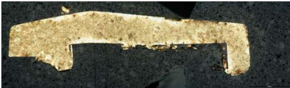
FIGURE 65 : MICROGRAPHIE OBTENUE APRES ATTAQUE A L'EAU REGALE D'UNE PIECE (POUDRE CLASSIFIEE) FRITTEE SELON LE CYCLE DE REFERENCE ARRETE AU DEBUT DU PALIER DE FRITTAGE ET SOUS UN DEBIT DE 25ML/S D'HYDROGENE PUR
