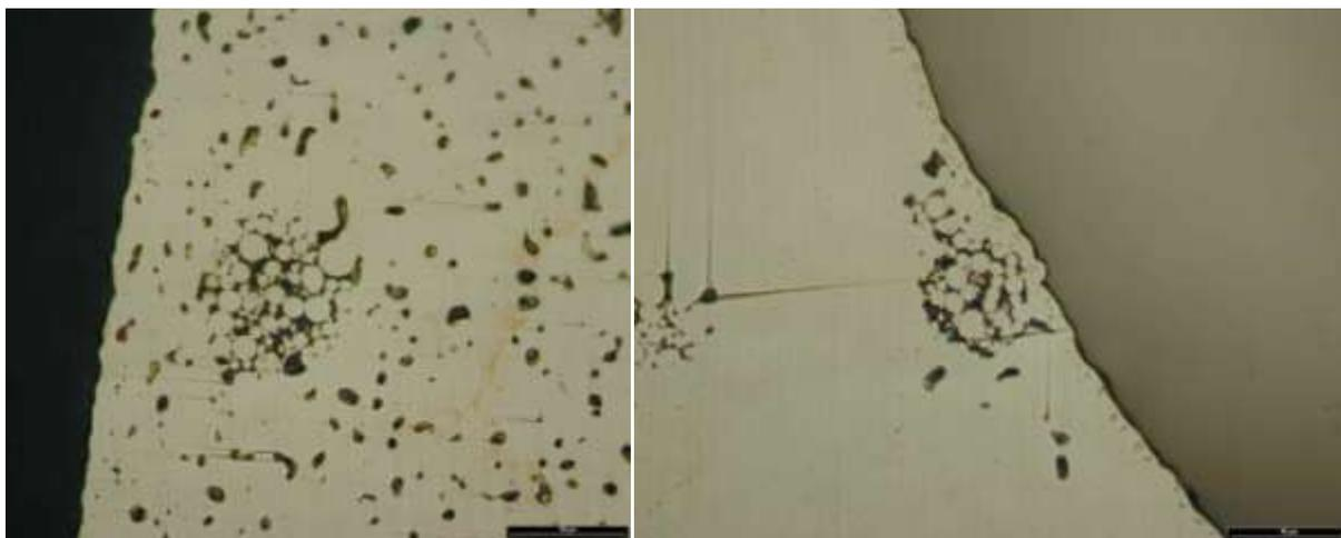
FIGURE 97: PIÈCE FRITTÉE AVEC LE CYCLE DE RÉFÉRENCE SANS POST TRAITEMENT (A GAUCHE) ET AVEC POST TRAITEMENT (A DROITE)
