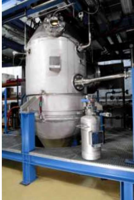
FIGURE 6 : PHOTO D'UNE TOUR D'ATOMISATION AU GAZ (LERMPS) <sup>[39]</sup>
