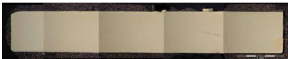
FIGURE 95: PASTILLE FRITTEE AVEC LE CYCLE DE REFERENCE SANS POST TRAITEMENT
