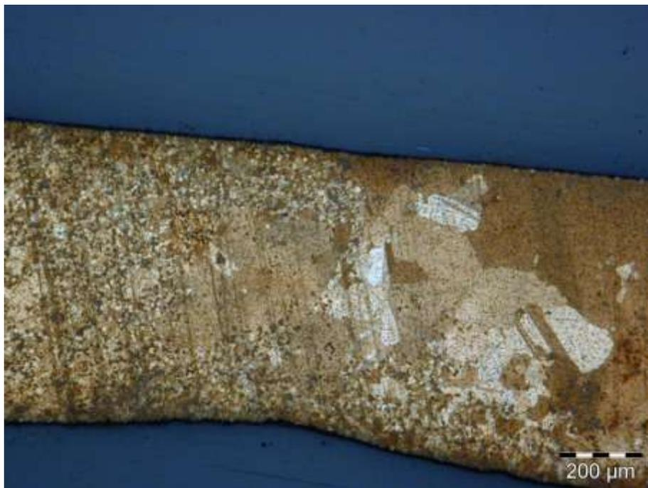
FIGURE 34 : MICROSTRUCTURE D'UNE PIÈCE (POUDRE CLASSIFIÉE HILDERBRAND+FEEDSTOCK PARMACO) RÉALISÉE AVEC LE CYCLE CONSEILLÉ PAR PARMACO AVEC UN POST TRAITEMENT HIP
