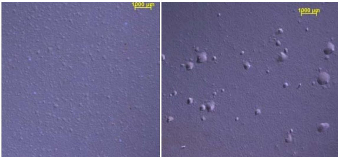
Figure 1.19: Optical microscopy observation of painted system after 1000 h immersion test. Adapted from [91].
