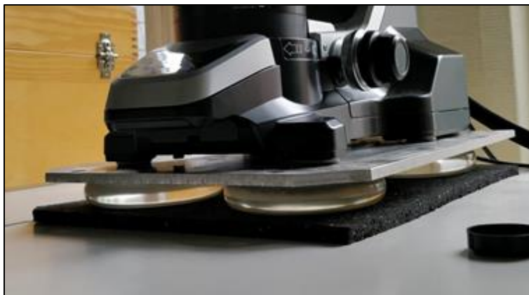
Figure 2.16: Photography of the anti-vibration setup for Keyence 3D microscope
