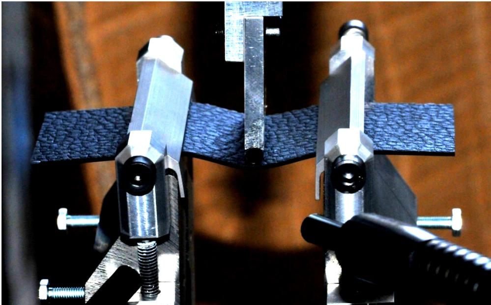
Figure 2.22: Top view of the experimental setup for SENB tests
