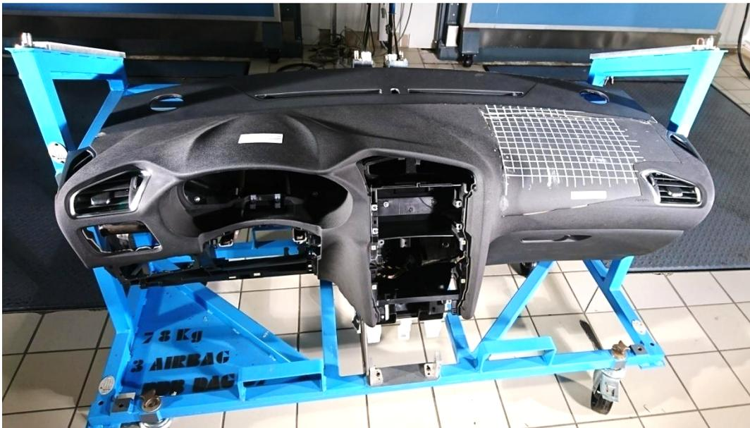
Figure 1.1: Dashboard before an airbag shot test. Grids of 34 cm x 26 cm sizes were set onto the passenger's airbag window so as to follow the deformation field and the crack progress during the test.
