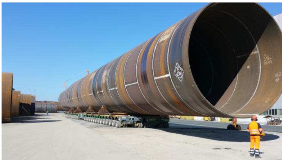
Fig. 2.7.: Fabricated monopile for Veja Mate offshore wind farm Windindustrie in Deutschland, 2016
