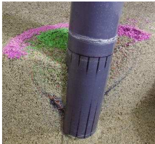
Fig. 5.8.: Photo of the subsidence cone and the sand convection cell formed around the monopile after a cyclic test (from Cuéllar, 2011)
