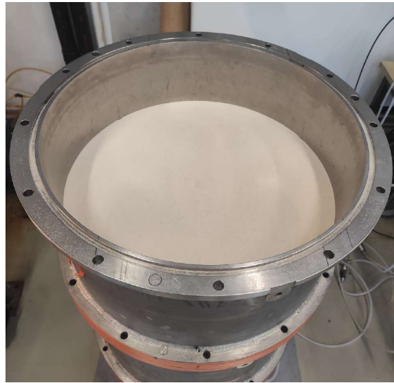
Fig. A.6.: Photo of chamber used to form the sand mass on monotonic and cyclic tests
