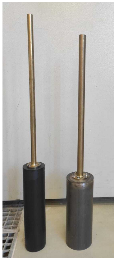
Fig. A.9.: Photo of scale models (monopile-substructure) M1 and M2
