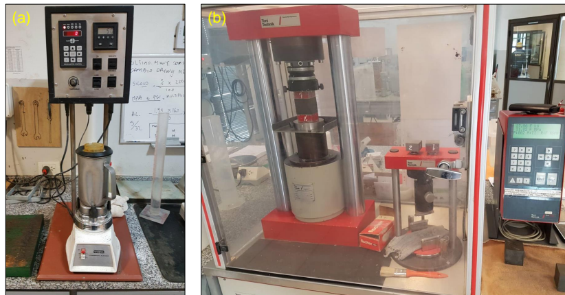
Fig. 3.2: (a) API mixer (b) uniaxial compression test.
