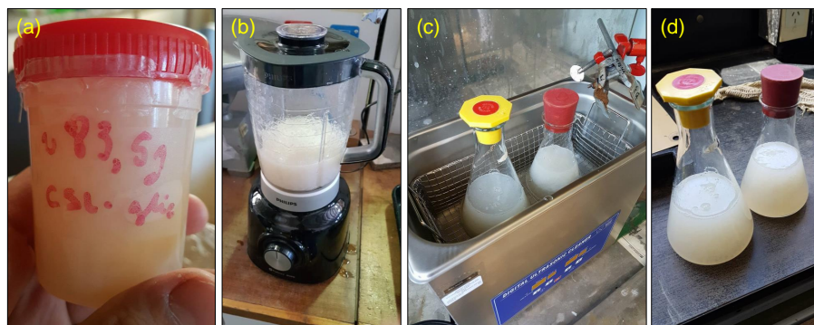
Fig. 3.1: (a) BNC in sealed jars, (b) BNC wet-grounded and mixed together with additional water, (c) ultrasonic bath, and (d) BNC final additive.
