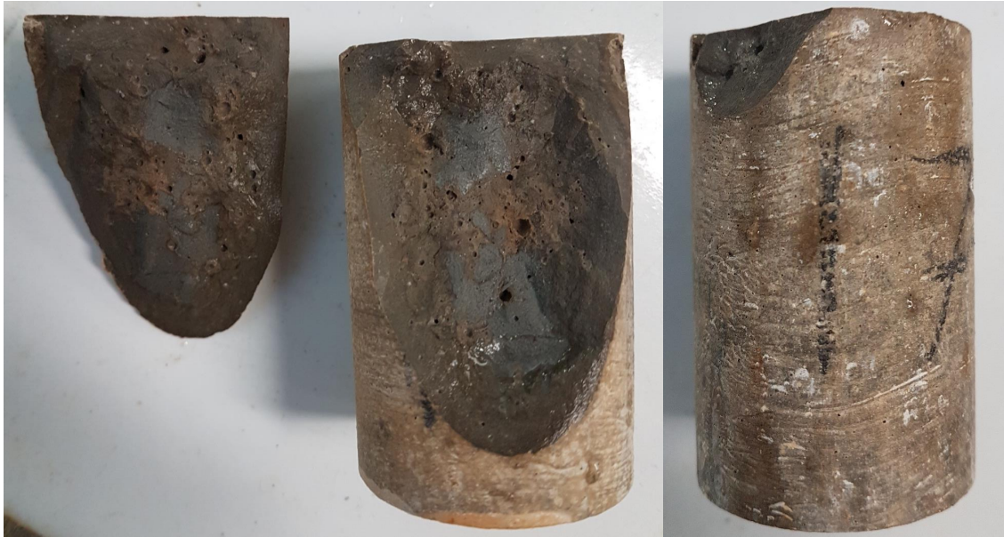
Fig. 4.37: Cracks in samples of cement cured under unfavorable conditions and carbonated for 120 days.
