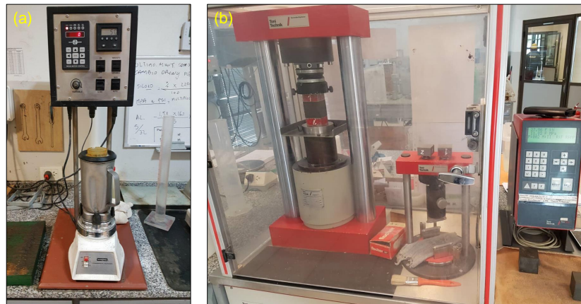
Fig. 3.2: (a) API mixer (b) uniaxial compression test.
