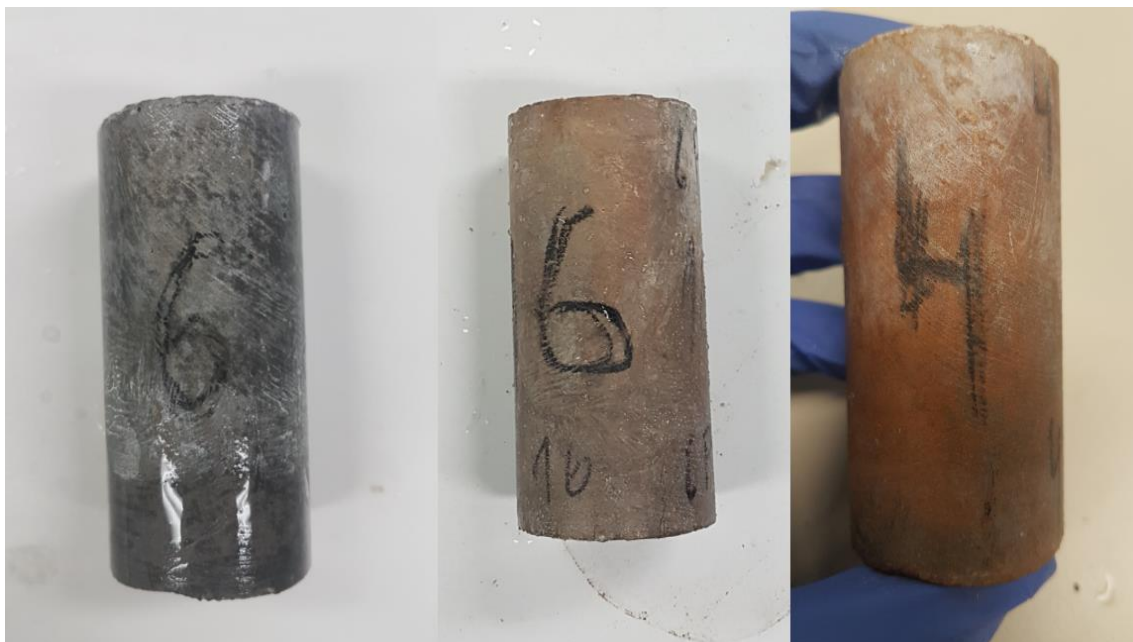
Fig. 4.15: Variation in the coloration of carbonated samples at 30 and 120 days.
