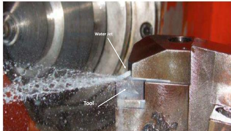
Figure II.14 – Illustration of the High Pressure machining approach (Braham Bouchnak, 2010)
