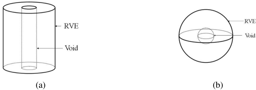
Figure 1.24. Cylindrical (left) and spherical (right) geometries for the void and the RVE considered by Gurson (1977).
