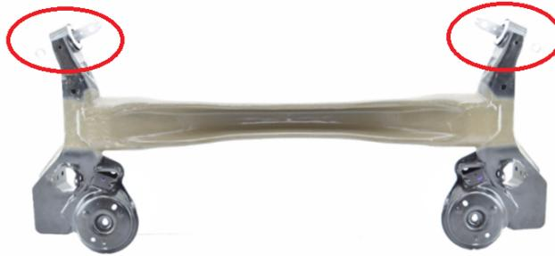
Figure 5.15: Twist beam axle with highlighted bushings.
