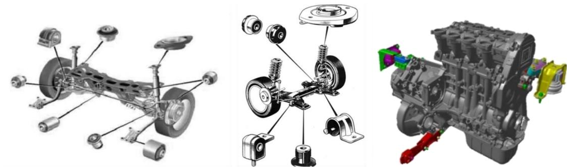
Figure 28: Localization of elastomeric bushings and mounts in front suspension, rear suspension and engine suspension.
