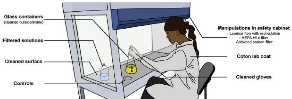
Fig. 2. Representation of basic precautions to avoid sample contamination in the context of MP load analysis.
