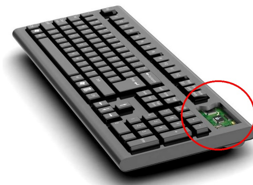
Figure 5.12: Already trapped keyboard with an embedded malicious printed circuit board.
