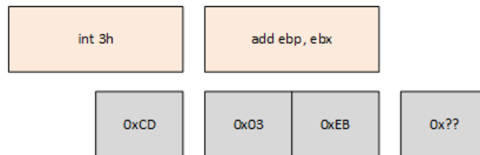
Figure 3.5: Illustration of the incorrect disassembling of "int 3h" by Windbg.
