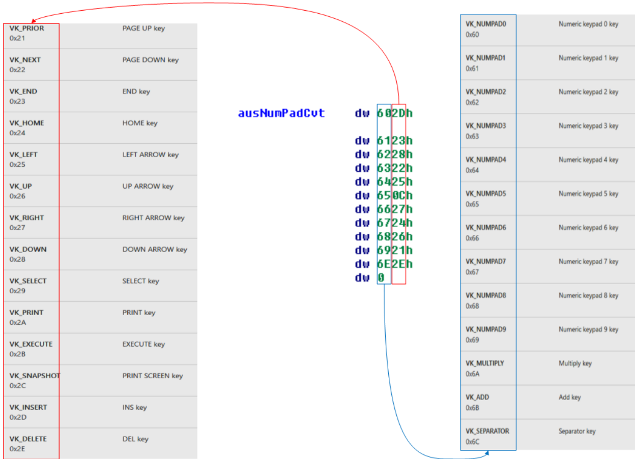
Figure 4.101: Illustration about the translation performed in xxxNumpadCursor routine with ausNumPadCvt table from win32kbase.sys.
