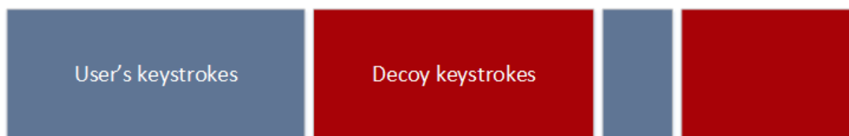
Figure 5.21: Illustration of the sequences between user’s keystrokes and decoyed ones. It is not hard to find user’s relevant information inside log files for keylogger’s managers.
