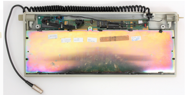
Figure 4.6: Bottom cover removed to get access to the metal bar that makes contact between the hammers and the PCB underneath.
