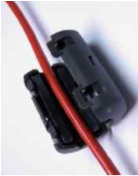
Figure 5.13: Example of contact less keylogger from [10].
