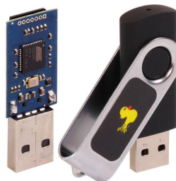
Figure 4.16: Rubber ducky dongle used to emulate a keyboard with pre-recorded sequences of keystrokes. The technologies behind this type of device are direct applications of USB and HID protocols.
