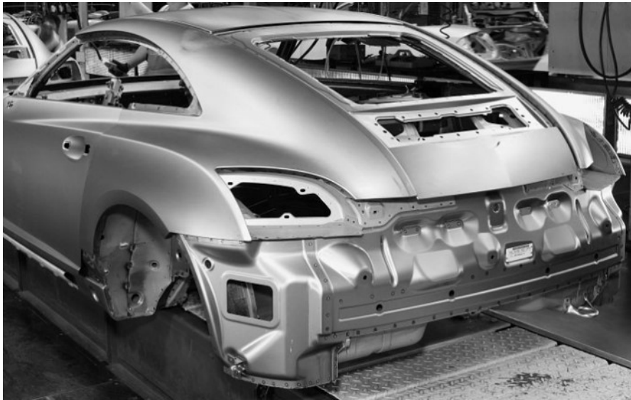
Figure 1.2 – A back-end car structure primarily assembled with spot welds from [Don+05].
