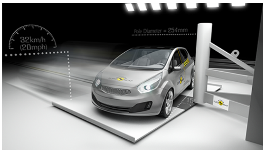
Figure 1.1 – EuroNCAP pole-impact assessment simulates lateral chocs with trees or poles on a roadside. Image from [Eur20b]. The use case later presented in chapter 3 is related to this scenario.
