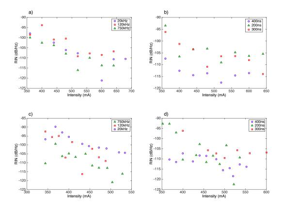
Figure 2.17: a) ARMEXEL RIN evolution with current for 300 ns pulses at 100 kHz at several measurement frequencies. b) ARMEXEL RIN evolution with current at a repetition rate of 100 kHz measured at 20 kHz for several pulse widths. c) PICOLAS RIN evolution with current for 300 ns pulses at 100 kHz at several measurement frequencies. d) PICOLAS RIN evolution with current at a repetition rate of 100 kHz measured at 20 kHz for several pulse widths.
