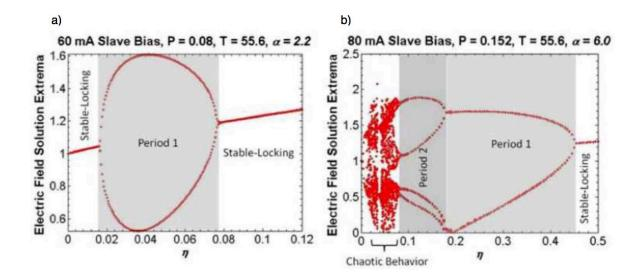
Figure 6.7: Examples of bifurcation diagrams depending on the slave laser parameters. Here the normalized parameters have the same definition as for optical feedback (courtesy of [187]).
