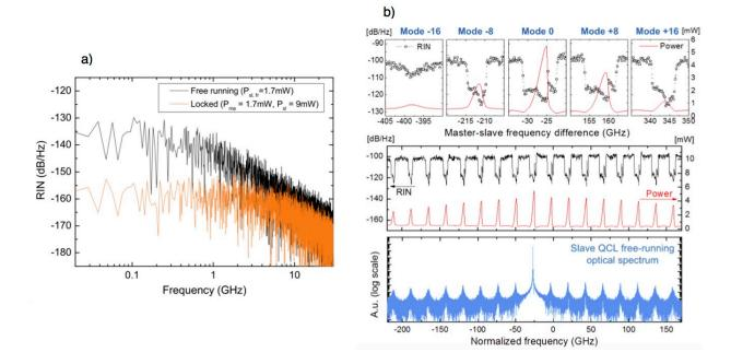
**Figure 6.10:** a) Numerical RIN reduction with optical injection (courtesy of [191]). b) Experimental RIN and power evolution with the frequency detuning: when one of the slave laser mode is locked on the master frequency, the RIN is reduced and the power increased (courtesy of [60]).
