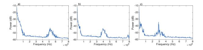
**Figure 4.19:** Experimental electrical spectral at  $f_{ext} = 3.1\%$  and P = 0.02 for several external cavity lengths, showing both the external cavity frequency and a low frequency corresponding to LFF. a)  $L_{ext} = 25$  cm. b)  $L_{ext} = 35$  cm. c)  $L_{ext} = 45$  cm.
