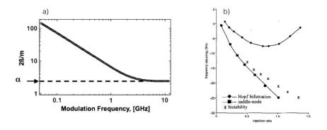
**Figure 2.8:** a) Measurement of the  $\alpha$ -factor using FM-AM ratio (courtesy of [42]). b) Minimum of the Hopf bifurcation of a laser under optical injection, giving a LEF of 3.2 (courtesy of [43]).
