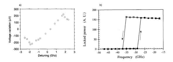
**Figure 6.5:** a) Voltage evolution with the detuning, showing the locking range. b) Influence of the detuning on the optical power at constant injection strength. (Courtesy of [178]).
