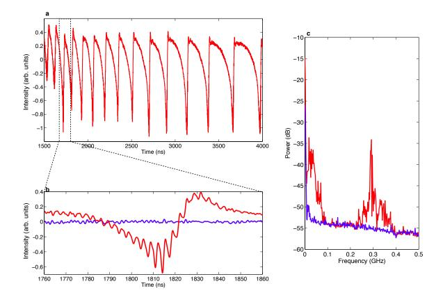
Figure 4.18: Typical experimental results, for P = 0.02,  $L_{ext} = 45$  cm and  $f_{ext} = 3.13\%$ . a) Time trace with slow fluctuations. b) Zoom on one slow period, a faster fluctuation appears at the external cavity frequency (in red), comparison with the free-running case (in blue). c) Electrical spectra that confirms the appearance of the external cavity frequency and of a slower frequency (in red), comparison with the free-running case (in blue).
