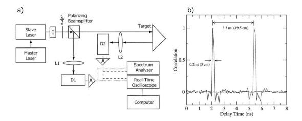
**Figure 3.20:** a) Experimental setup of a chaotic LIDAR. In this case, the chaos is obtained from optical injection. b) Experimental result, showing a precise measurement of the 50 cm separated targets, with a range resolution of 3 cm (courtesy of [119]).
