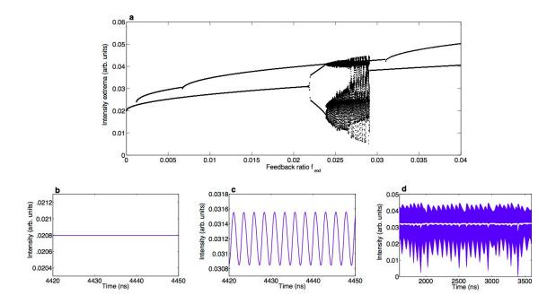
**Figure 4.22:** Numerical bifurcation diagram for P = 0.02 and  $L_{ext} = 35$  cm, and associated time series. a) Numerical bifurcation diagram. b) Time trace for  $f_{ext} = 0.11\%$ , showing stable signal. c) Time trace for  $f_{ext} = 2.14\%$ , showing oscillations at the external cavity frequency. d) Time trace for  $f_{ext} = 2.59\%$ , showing both LFF and oscillations at the external cavity frequency.
