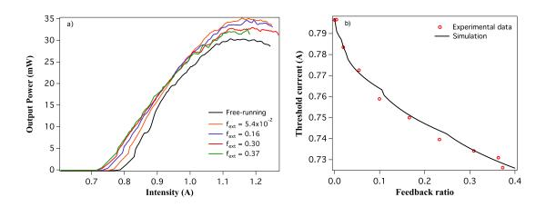
**Figure 4.12:** Impact of optical feedback on the 4 mm  $\times$  6  $\mu$ m FP QCL L-I curves. a) L-I characteristic curves for several feedback ratios, with an external cavity length of 13 cm. b) Experimental and numerical threshold reduction as a function of the feedback ratio.
