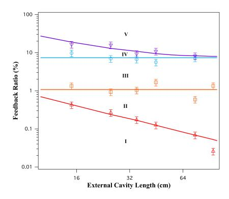
Figure 4.16: Feedback cartography of the different regimes of the DFB QCL as a function of the external cavity length and the feedback ratio, measured at 10°C for a bias current of 435 mA.
