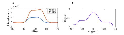
Figure 5.14: a) Evolution of the near-field profile with the bias voltage of a 14  $\mu$ m QCL based on a different design, evidencing strong beam steering. b) Deteriorated far-field of the laser at high bias current.
