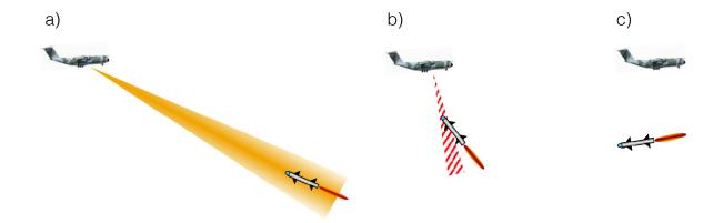
**Figure 1.3:** Scenario of optical countermeasure. a) A missile is detected while tracking the plane heat signature. b) A strong mid-infrared signal is sent from the plane to jam the missile. c) The missile trajectory is deviated.
