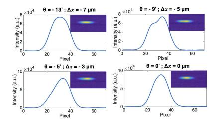
Figure 5.13: Near-field at the facet for the 14  $\mu$ m QCL based on the previously described design, for different feedback angle.
