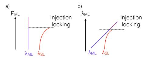
**Figure 6.2:** Schematic of injection locking. a) Evolution of the slave wavelength  $\lambda_{SL}$  as a function of the injected power. b) Evolution of the slave wavelength  $\lambda_{SL}$  as a function of the master wavelength  $\lambda_{ML}$ .
