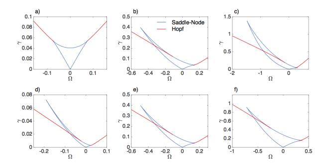
**Figure 6.11:** Analytical simulations of the 12  $\mu$ m Fabry-Perot QCL subject to optical injection. First row: constant bias current I = 1.5 A with a)  $\alpha = 0$ , b)  $\alpha = 1.5$  and c)  $\alpha = 3$ . Second row: fixed  $\alpha = 1.5$  and d) I = 1.25 A, e) I = 1.5 A, f) I = 2 A.
