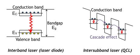
Figure 2.2: Intersubband transitions and cascade effect.
