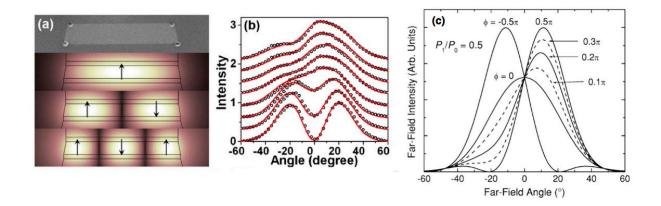
**Figure 5.8:** a) SEM picture of the laser facet and simulated TM0, TM1 and TM2. b) Measured (black dots) and fitted (red lines) far-fields at different bias currents. Courtesy of [165]. c) Simulated far-field in case of equal power coupling between TM0 and TM1 for various phase difference (courtesy of [166]).
