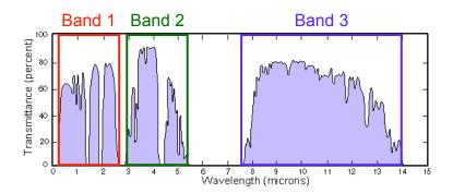
Figure 1.1: Atmospheric optical windows.
