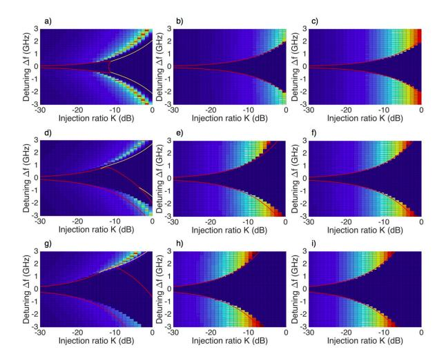
**Figure 6.13:** Numerical simulations of the signal intensity as a function of the injection ratio and detuning, superimposed on the analytical solutions (red for Saddle-Node and yellow for Hopf curves) for the 12  $\mu$ m Fabry-Perot QCL subject to optical injection. First row:  $\alpha = 0$  with a) I = 1.25 A, b) I = 1.5 A, c) I = 2 A. Second row:  $\alpha = 1.5$  with d) I = 1.25 A, e) I = 1.5 A, f) I = 2 A. Third row:  $\alpha = 3$  with g) I = 1.25 A, h) I = 1.5 A, i) I = 2 A.
