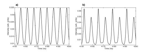
Figure 3.11: Time traces corresponding to Figure 3.10 a. a) Period 1, for  $\eta = 2 \times 10^{-4}$ . b) Period 2, for  $\eta = 8 \times 10^{-4}$ .
