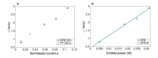
Figure 4.9: a)  $\alpha$ -factor evolution as a function of the normalized current and comparison between the two methods at 10°C. b)  $\alpha$ -factor evolution as a function of the emitted power for the DFB QCL.
