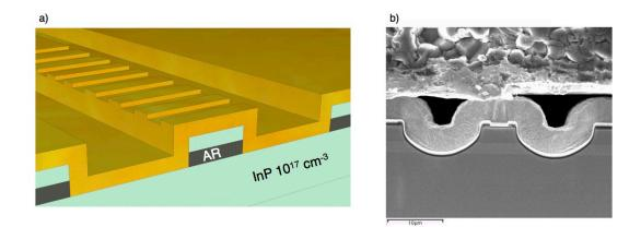
**Figure 2.10:** a) Schematic and b) SEM picture of the DBF QCL under study. The active region, labeled 'AR' in a), appears in b) in lighter gray.
