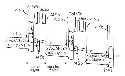
Figure 1.6: Schematic of the first ICL (courtesy of [10]).
