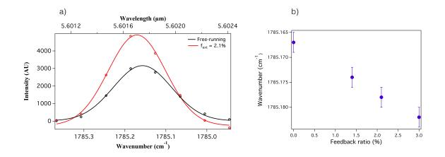
Figure 4.7: Wavelength evolution of the QCL under optical feedback. a) Optical spectra and gaussian fits without feedback and with low feedback  $f_{ext} = 2.1\%$ . b) Experimental wavelength shift as a function of the feedback ratio.
