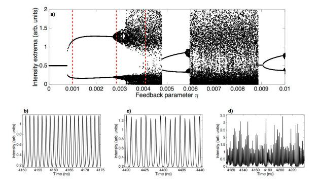
Figure 3.9: a) Numerical bifurcation diagram for T = 1700, P = 0.5,  $\theta = 500$  (L<sub>ext</sub>  $\approx 30$  cm) and  $\alpha = 3$ . b) Corresponding time trace for  $\eta = 0.001$ . c) Time trace for  $\eta = 0.0027$ . d) Time trace for  $\eta = 0.0042$ .
