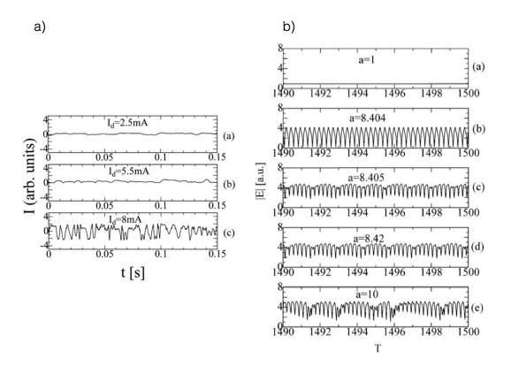
**Figure 3.19:** a) Experimental time traces of a class A laser for several feedback parameters a (equivalent to k) showing the appearance of LFF (courtesy of [111]). b) Numerical time traces of a class A for several feedback parameters showing oscillations at the external cavity frequency followed by LFF (courtesy of [112]).
