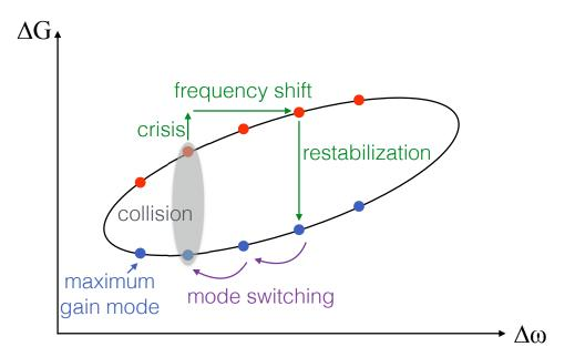
Figure 3.16: Schematic of the scenario leading to LFF. In blue circles, stable external cavity modes, and in red circles, unstable antimodes.
