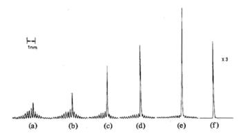
**Figure 6.4:** Optical spectra of a laser diode as a function of the injected power (courtesy of [172]). a) Free-running case. b)  $P_{inj} = -49.5$  dBm. c)  $P_{inj} = -42.5$  dBm. d)  $P_{inj} = -39.5$  dBm. e)  $P_{inj} = -29.5$  dBm. f)  $P_{inj} = -22.5$  dBm.
