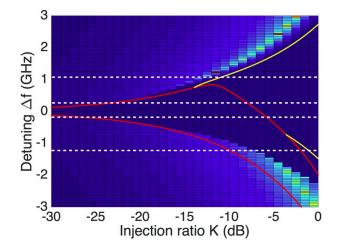
Figure 6.15: Measurement points (in dashed lines) for the numerical time traces of the  $12\mu$ m QCL under optical injection represented in Figure 7.22 for  $\alpha = 1.5$  and I = 1.25 A.
