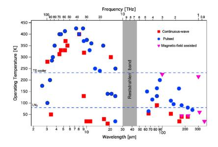
Figure 2.1: QCL performances reported in the literature, as a function of wavelength and operating temperature (courtesy of [19]).
