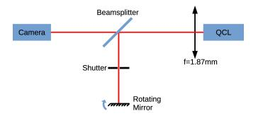
Figure 5.1: Experimental setup for BA-QCLs.
