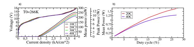
**Figure 5.5:** a) LIV curves at 3% duty cycle for temperatures from  $10^{\circ}$ C to  $40^{\circ}$ C. b) Evolution of the mean power with duty cycle at  $20^{\circ}$ C and  $40^{\circ}$ C
