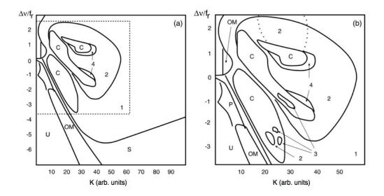
Figure 6.8: Experimental locking map, presenting the complex dynamics of a laser subject to optical injection. The dashed area in a) is represented in b) (courtesy of [188]).
