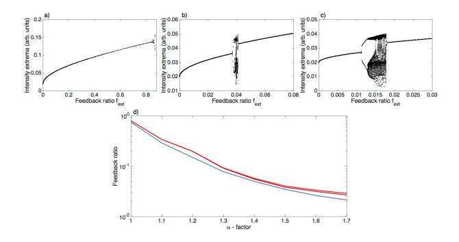
**Figure 4.23:** Influence of the  $\alpha$ -factor on the bifurcation diagram for P = 0.02 and  $L_{ext} = 35$  cm. a) Numerical bifurcation diagram for  $\alpha = 1$ . b) Numerical bifurcation diagram for  $\alpha = 1.5$ . c) Numerical bifurcation diagram for  $\alpha = 2$ . d) Evolution of the Hopf point (in blue) and of the lower and upper limits of the LFF area (in red) as a function of the  $\alpha$ -factor.
