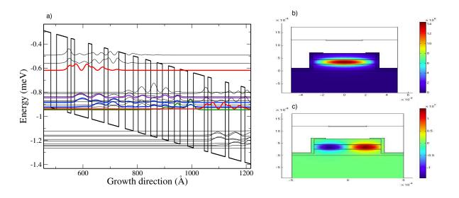
Figure 2.11: a) Wave functions of the QCL structure under study, simulated with METIS. In red, levels  $|3\rangle$  of two consecutive periods, in violet level  $|2\rangle$ , in blue level  $|1\rangle$  split into two phonon states, in green injector state. b) Fondamental mode TM0 simulation using COMSOL. c) TM1 simulation.
