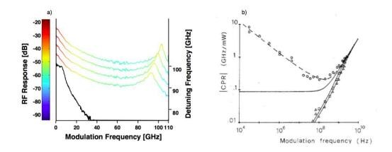
**Figure 6.6:** a) Improvement of the modulation bandwidth with optical injection, compared to the free-running case in black (courtesy of [182]). b) Chirp reduction with optical injection, compared to the free-running represented by circles (courtesy of [183]).
