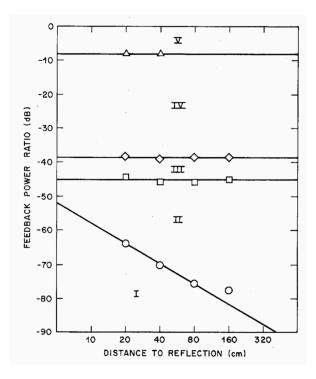
Figure 3.2: Cartography of optical feedback in a DFB quantum well laser (courtesy of [74]).
