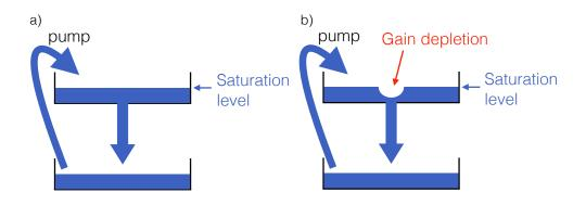
Figure 4.10: Gain saturation (a) versus gain compression (b).
