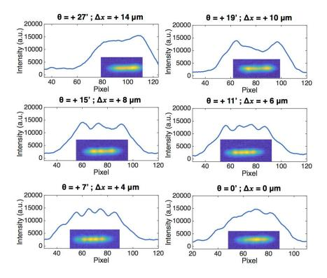
Figure 5.12: Near-field at the facet for the 32  $\mu$ m-wide QCL presenting a defect, for different feedback angle.
