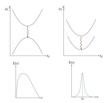
Figure 2.4: Comparison between interband laser (a) and QCL (b). The upper curves represent the place where the lasing transition takes place, and the lower ones show the energy density  $E(\nu)$ .
