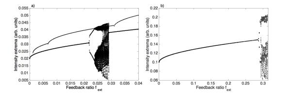
Figure 4.24: Influence of the bias parameter P on the bifurcation diagram for  $L_{ext} = 35$  cm and  $\alpha = 1.7$ . a) Numerical bifurcation diagram for P = 0.02. b) Numerical bifurcation diagram for P = 0.10.
