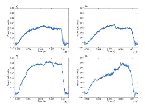
**Figure 5.3:** Temporal power evolution with optical feedback. a) Free-running scenario. b) Decrease of the power. c) Increase of the power. d) Appearance of oscillations.
