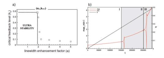
Figure 4.3: a) Critical feedback level for a THz QCL, which becomes very high when the  $\alpha$ -factor becomes small (courtesy of [130]). b) Numerical evolution when increasing the feedback coefficient k, showing mode switching (courtesy of [131]).
