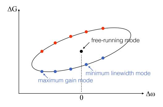
Figure 3.6: Ellipse of the feedback modes and anti-modes. In blue circles, stable external cavity modes, and in red circles, unstable antimodes.
