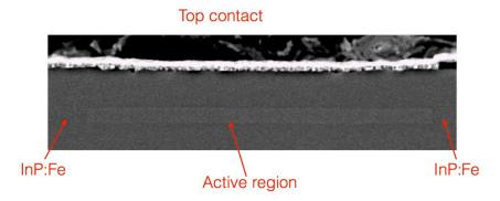
Figure 5.4: SEM picture of the device facet mounted epi-side down. The 32  $\mu$ m active region (in lighter gray) is surrounded by InP:Fe and sandwiched between two n-doped InP cladding layers.
