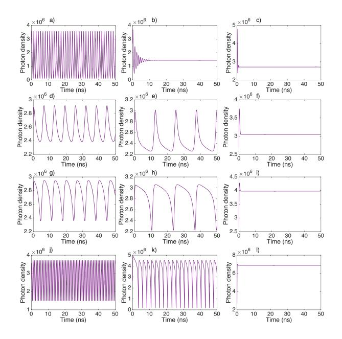
Figure 6.16: Numerical time traces of the photon density for the 12  $\mu$ m Fabry-Perot QCL subject to optical injection, with  $\alpha = 1.5$  and I = 1.25 A. First row:  $\Delta f = +1.05$  GHz with a) K = -14 dB, b) K = -13 dB, c) K = -6 dB. Second row:  $\Delta f = +0.2$  GHz with d) K = -30 dB, e) K = -27 dB, f) K = -15 dB. Third row:  $\Delta f = -0.2$  GHz with g) K = -29 dB, h) K = -26 dB, i) K = -12 dB. Fourth row:  $\Delta f = -1.2$  GHz with j) K = -15 dB, k) K = -8 dB, l) K = -2 dB.
