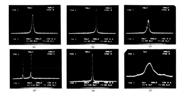
**Figure 3.3:** Example of optical spectra for a VCSEL at different feedback ratios, representative of the regimes (courtesy of [75]). a) Free-running laser. b) and c) Regime I, at  $f_{ext} = -72$  dB for several phase conditions. d) Regime II, at  $f_{ext} = -52$  dB. e) Regime III, at  $f_{ext} = -38$  dB. f) Regime IV, at  $f_{ext} = -23$  dB.
