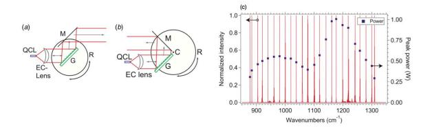
**Figure 4.1:** a,b) External-cavity QCL in different configurations. c) Achievable wavelengths by tilting the grating. (Courtesy of [127]).
