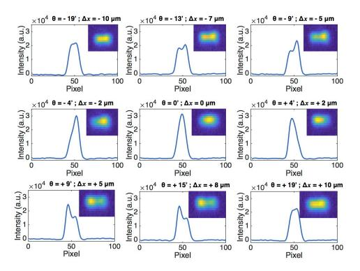
Figure 5.15: Impact of optical feedback on a 14  $\mu$ m QCL based on a different design presenting strong beam steering.
