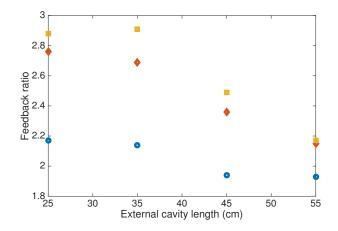
Figure 4.25: Influence of the external cavity length  $L_{ext}$  on the bifurcation diagram for P = 0.02 and  $\alpha = 1.7$ . In blue circles, occurrence of the first Hopf bifurcation. In red diamonds, appearance of the LFF. In yellow squares, restabilization.
