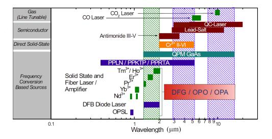
Figure 1.4: Main infrared sources and their emission range.
