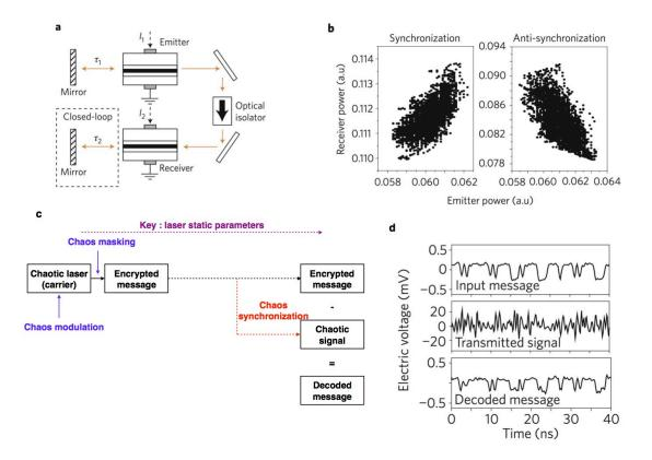
**Figure 3.21:** Chaos-based communications. a) Setup for chaos synchronization. b) Experimental results showing synchronization and anti-synchronization. c) Principle of chaos-encrypted communications. d) Example of chaos-based communications. (a, b and d are courtesy of [118])
