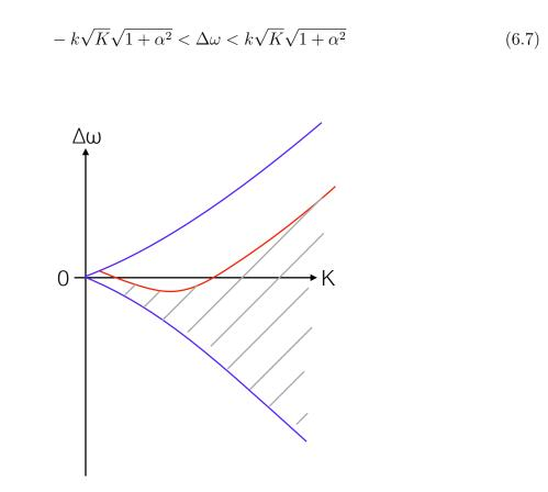
**Figure 6.3:** Typical locking map of a laser diode. In blue, Saddle-Node bifurcations. In red, Hopf bifurcation. In dashed gray, stable locking region.
