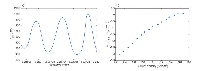
Figure 2.14: a) DFB transmitted intensity as a function of the FP refractive index, for a current density in the Fabry-Perot laser of  $3.35 \text{ kA/cm}^2$ . b) Fabry-Perot QCL modal gain evolution as a function of the bias current below threshold, at constant DFB laser operating conditions 589 mA and 9.8 V.
