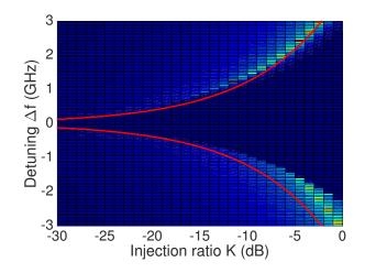
Figure 6.14: Influence of  $\eta$  on the locking map for the 12  $\mu$ m QCL with I = 1.25 A and  $\alpha = 1.5$ . The conversion efficiency is taken into account in the numerical calculation but taken to  $\eta = 1$  in the analytial curves.
