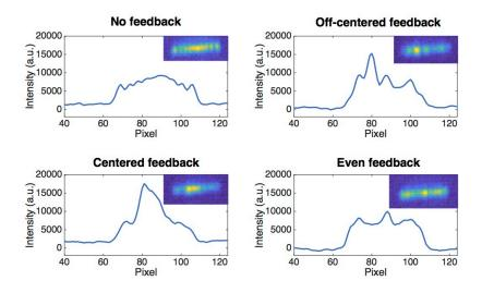
Figure 5.2: Near-field at the laser facet for several feedback angle. Plots in inset correspond to the near-field recorded on the camera.
