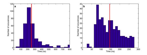
Figure 4.20: Statistical distributions of the slow fluctuations, for  $L_{ext} = 35$  cm. a) P = 0.02 and  $f_{ext} = 3.5\%$ . b) P = 0.10 and  $f_{ext} = 0.11$ . In both cases, the red line indicates the average value.
