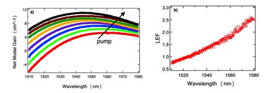
**Figure 2.7:** Illustration of the Hakki-Paoli method for a quantum dot laser. a) Gain shift as a function of the sub-threshold bias current. b) Deduced  $\alpha$ -factor. (Courtesy of [40]).
