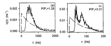
**Figure 3.17:** Statistics of the period between two consecutive drop-outs. a)  $\tau_{ext} = 10$  ns and P = 1.28. b)  $\tau_{ext} = 1$  ns and P = 3.31. (P<sub>1</sub> = 1) (courtesy of [106]).
