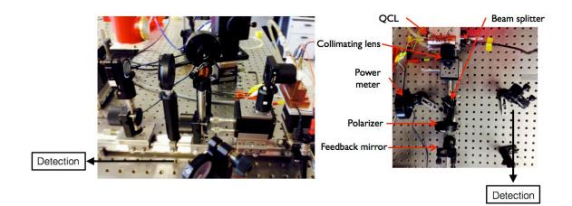
Figure 4.6: Experimental setup for optical feedback in QCLs.
