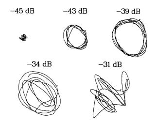
Figure 3.13: Experimental phase diagrams showing the route to chaos (courtesy of [94]).
