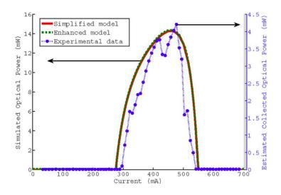
Figure 2.5: Comparison between complete set of equations in green, and simplified model in red (courtesy of [28]).
