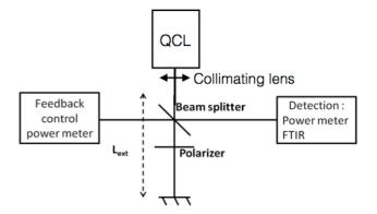
Figure 4.4: Schematic of the experimental setup for optical feedback in QCLs.
