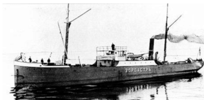
Figure 1.1: Photograph of the Zoroaster [25], first tanker. length: 54 m, capacity: 240 tons
