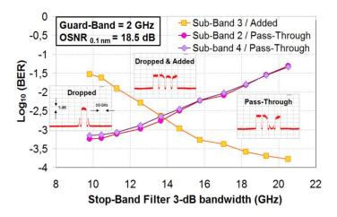
Figure 4-8: BER versus 3-dB BW of the OSBF for the sub-bands 2, 3 & 4 and a GB = 2 GHz. In insets, the spectra of the signals at the optimum.
