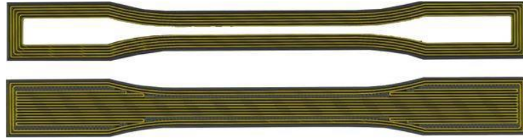
Fig 46. Cross-section view of concentric (top) and isotropic (bottom) infills [58]
