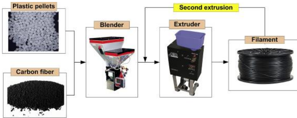
Fig. 50. Manufacturing the feedstock filament for the FFF process [55]
