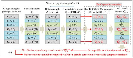
Figure 4.15 – Conceptual diagram of determining the wave type existing in the metallic-composite laminate [Al/0/90/Al/90/0/Al] at the wave propagation angle (a)  $\theta = 0^{\circ}$ , (b)  $\theta = 45^{\circ}$  and (c)  $\theta = 45^{\circ}$  for Pant's pseudo correction.
