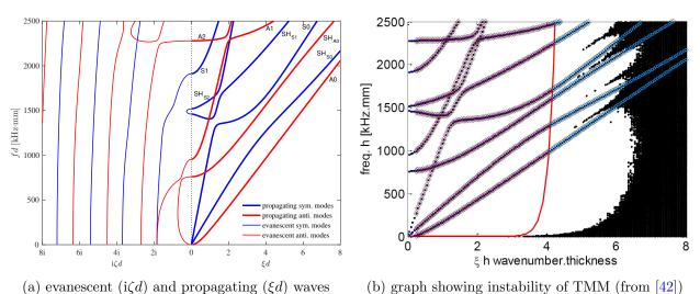
(a) oralloscond (i, a) and propagating (a) waves (b) grad
