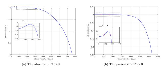
Figure 6.3 – The typical  $\Delta - v$  relation showing (a) the absence of  $\Delta > 0$  and (b) the presence of  $\Delta > 0$  in a narrow phase velocity range.
