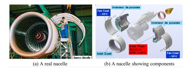
Figure 1.3 – Picture of a nacelle [3]
