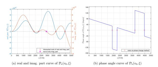
Figure 6.18 – Function curve of the symmetric modes of dispersion equation  $\mathcal{D}_s(v_0,\xi)$  for a triclinic material at  $v_0 = 4000 \text{ m/s}$ .
