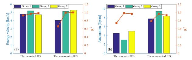
Figure 7.17 – Comparison between the mounted and unmounted IFS for (a) energy velocity and (b) attenuation coefficient at 100 kHz. In the two subfigures, the bars relate to the left y-axis and the lines correlate to the right y-axis.
