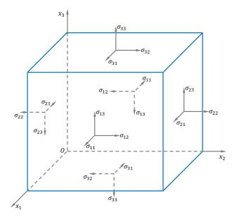
Figure 2.1 – The stress state of a cubic element of a solid material.
