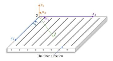
Figure 2.4 – The schematic diagram of bulk wave propagation.
