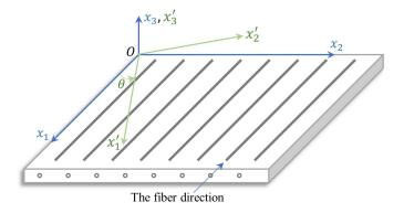
Figure 2.2 – The schematic diagram of a composite lamina.
