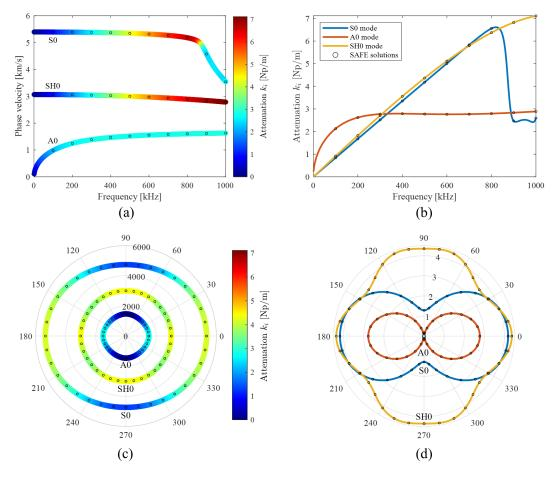
Figure 7.14 – For the unmounted FCS, HR model's prediction of (a) dispersion curve of phase velocity at  $\theta = 180^{\circ}$ , (b) dispersion curve of attenuation coefficient at  $\theta = 180^{\circ}$ , (c) polar plot of phase velocity [m/s] at f = 500 kHz, (d) polar plot of attenuation coefficient [Np/m] at f = 500 kHz. The open circles in the four subfigures are the solutions computed by SAFE method.
