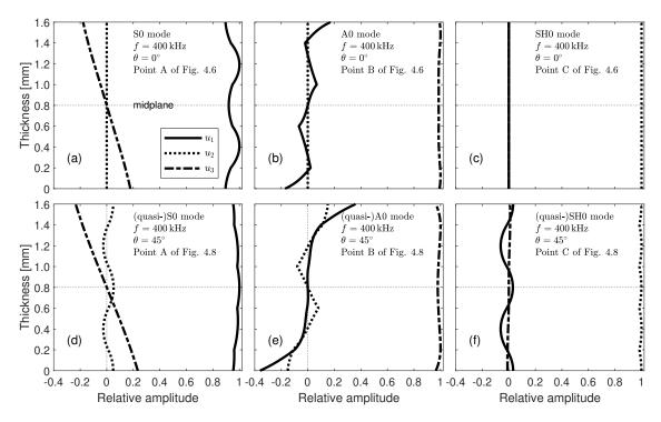
Figure 4.9 – Displacement mode shapes of the cross-ply laminate for  $\theta = 0^{\circ}$  and 45° at f = 400 kHz.
