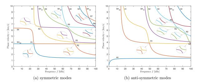
Figure 5.6 – Dispersion curves of the 400-layered aerospace laminate at  $\theta = 0^{\circ}$  direction.
