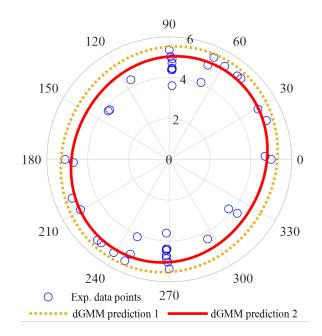
Figure 7.18 – Polar plot of S0 mode energy velocity [km/s] in the mounted IFS at 100 kHz. The contour of dGMM prediction 1 and dGMM prediction 2 are computed by using the  $(E_1, E_2, E_3)$  values 1 and 2 in Table 7.4, respectively.
