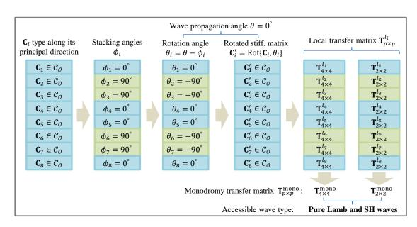
Figure 4.5 – Conceptual diagram of determining the wave type existing in the cross-ply laminate  $[(0/90)_s]_2$  at wave propagation angle  $\theta = 0^\circ$ .
