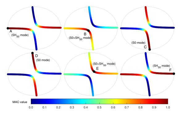
Figure 5.7 – MAC value tomography of displacement mode shapes in the region R1 of symmetric modes.
