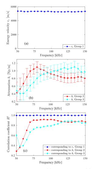
Figure 7.12 – The identified dispersion curves of (a) energy velocity, (b) attenuation coefficient and (c) correlation coefficient. These subfigures relate to the S0 mode propagating at  $0^{\circ}$  direction of the unmounted FCS.
