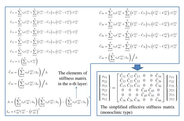
Figure 5.4 – Equations of ESM to compute the effective stiffness matrix [10].
