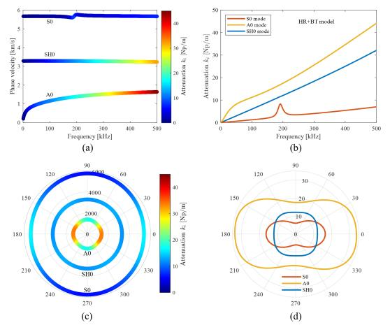
Figure 7.23 – For the unmounted IFS, HR+BT model's prediction of (a) dispersion curve of phase velocity at  $\theta = 90^{\circ}$ , (b) dispersion curve of attenuation coefficient at  $\theta = 90^{\circ}$ , (c) polar plot of phase velocity [m/s] at f = 200 kHz, (d) polar plot of attenuation coefficient [Np/m] at f = 200 kHz.
