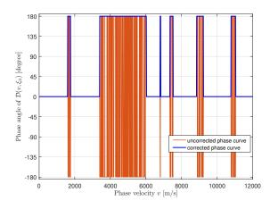
Figure 6.13 – Phase angle curve of  $\mathcal{D}_G(v, \xi_0 = 3000) = 0$  for the  $[0]_{50}$  unidirectional laminate.
