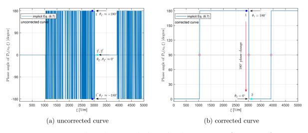
Figure 6.8 – Using phase change method to solve the equation  $\mathcal{D}_a(v_0 = 5000, \xi) = 0$ .
