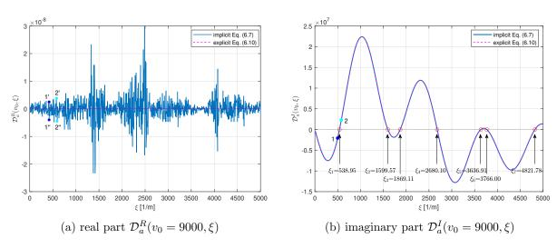
Figure 6.4 – Using bisection method to solve the equation  $\mathcal{D}_a(v_0 = 9000, \xi) = 0.$
