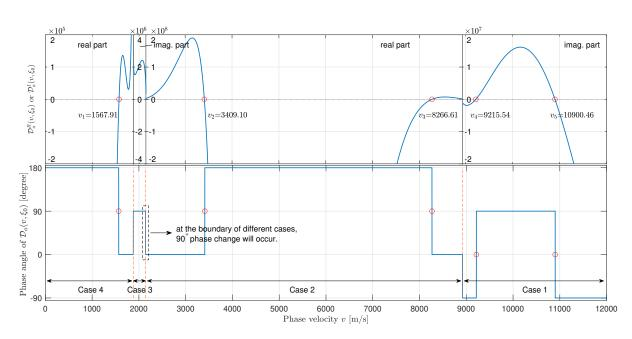
Figure 6.9 – Using bisection and phase change methods to solve the equation  $\mathcal{D}_a(v, \xi_0 = 1750) = 0$ . The small width of case 3 is caused by the degree of anisotropy.
