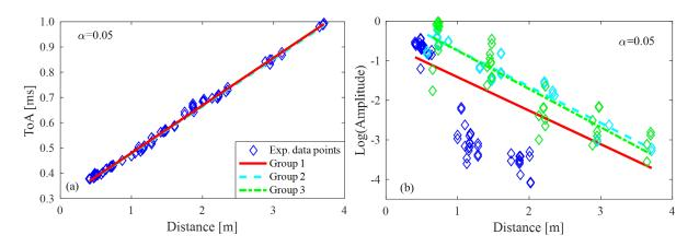
Figure 7.9 – Example of identifying (a) energy velocity and (b) attenuation coefficient via LR method at 100 kHz for the unmounted FCS. Both figures share the same legend and  $\alpha$  is used to give the confidence level with  $100(1 - \alpha)\%$ .
