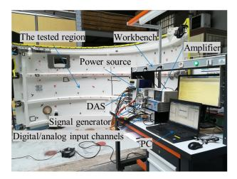
Figure 7.7 – The experimental setup of the unmounted FCS.
