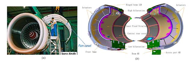
Figure 7.1 – The studied aircraft nacelles of an A380 plane for (a) fan cowl structure and (b) inner fixed structure.
