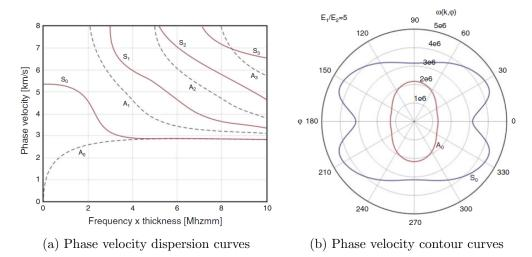
Figure 1.5 – Dispersion and directivity properties of guided waves velocity [4].
