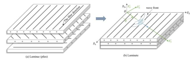
Figure 4.1 – A three-layered composite plate model  $[0/\theta/90]$ . The wave propagation direction is along the fiber direction of the middle layer.
