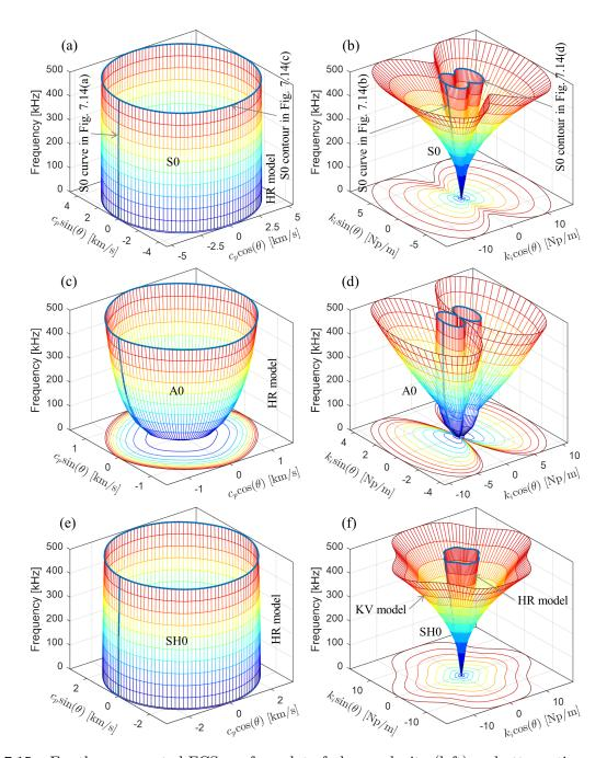
Figure 7.15 – For the unmounted FCS, surface plot of phase velocity (left) and attenuation coefficient (right): (a) and (b) S0 mode, (c) and (d) A0 mode, (e) and (f) SH0 mode. The inner and outer surfaces in subfigures (b)(d)(f) correspond to HR and KV models, respectively.
