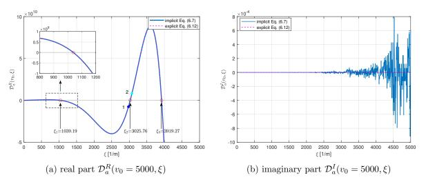
Figure 6.6 – Using bisection method to solve the equation  $\mathcal{D}_a(v_0 = 5000, \xi) = 0.$
