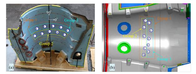
Figure 7.16 – The transducers layout of IFS for (a) the unmounted case and (b) the mounted case on an instrumented A380 plane.
