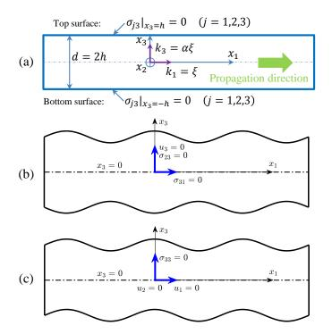
Figure 3.1 – Wave propagation model of a single-layered plate showing (a) boundary condition, (b) symmetric condition and (c) anti-symmetric condition.
