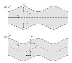
Figure 1.7 – Symmetric and anti-symmetric mode shapes of Lamb waves [4].
