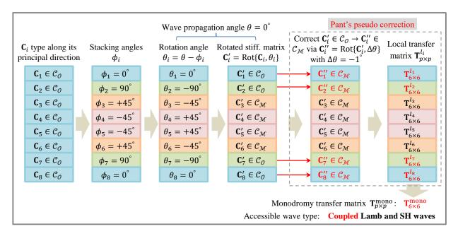
Figure 4.14 – Conceptual diagram of Pant's pseudo correction to deal with the incompatibility issue of the quasi-isotropic laminate  $[0/90/ + 45/ - 45]_s$  when  $\theta = 0^\circ$ .
