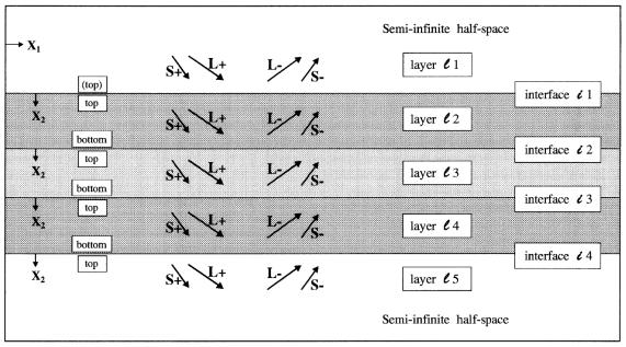
Example, using three-layer plate with semi-infinite half-spaces.
