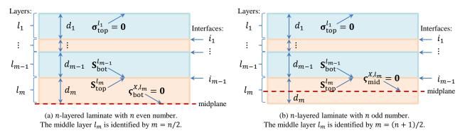
Figure 5.5 – A symmetric laminate showing only the upper half layers. In the SC  $\varsigma_{\text{bot}}^{X,l_m}$  and  $\varsigma_{\text{mid}}^{X,l_m}$ , the superscript X = s and a represent the symmetric and anti-symmetric condition, respectively.
