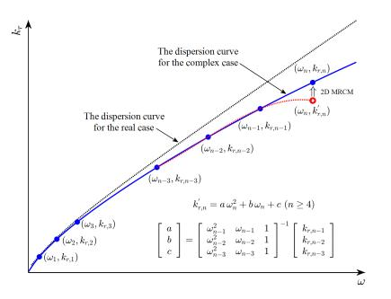
Figure 7.3 – The schematic diagram of the curve tracing technique.
