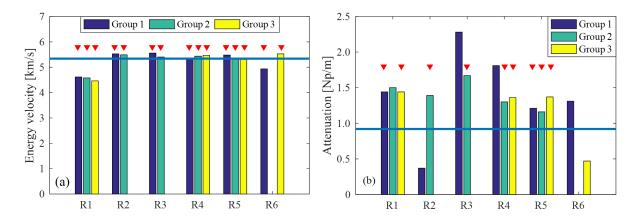
Figure 7.11 – Bar chart to display regression results of (a) energy velocity and (b) attenuation coefficient via LR method for the mounted FCS at 100 kHz. The horizontal line represents the reference value of the unmounted FCS, and the triangles denote that the marked bars correspond to a  $R^2$  larger than 0.7.
