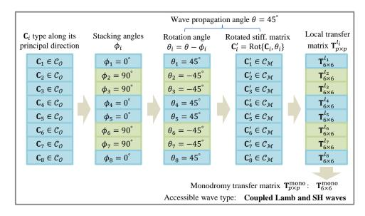
Figure 4.7 – Conceptual diagram of determining the wave type existing in the cross-ply laminate  $[(0/90)_s]_2$  at wave propagation angle  $\theta = 45^{\circ}$ .
