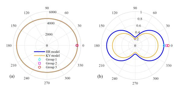
Figure 7.10 – Polar plot of S0 mode of (a) energy velocity [m/s] and (b) attenuation coefficient [Np/m] at 100 kHz for the unmounted FCS. Both subfigures share the same legend.
