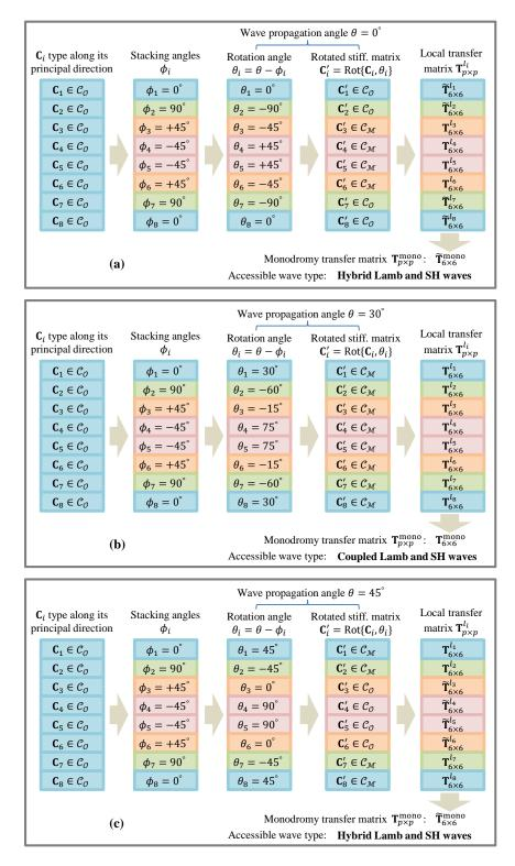
Figure 4.11 – Conceptual diagram of determining the wave type existing in the quasi-isotropic laminate  $[0/90/+45/-45]_{\rm s}$  at the wave propagation angle (a)  $\theta = 0^{\circ}$ , (b)  $\theta = 30^{\circ}$ , (c)  $\theta = 45^{\circ}$ .
