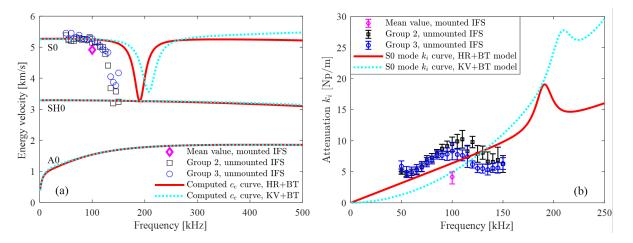
Figure 7.20 – Comparison between the computed and experimentally identified dispersion curves of (a) energy velocity and (b) attenuation coefficient for the unmounted IFS at  $\theta = 0^{\circ}$ .
