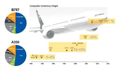
Figure 1.2 – Increasing usage of composite materials in aircraft structures over the past 40 years [2].
