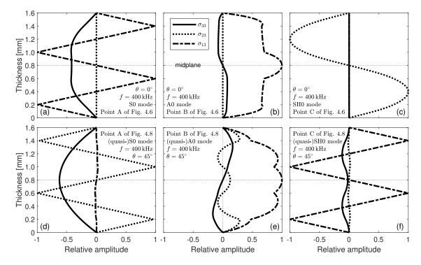
Figure 4.10 – Stress mode shapes of the cross-ply laminate for  $\theta = 0^{\circ}$  and  $45^{\circ}$  at f = 400 kHz.
