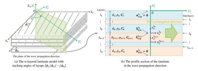
Figure 4.2 – Guided wave propagation model in a *n*-layered composite laminate.
