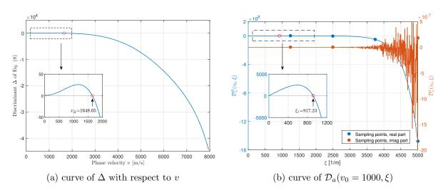
Figure 6.15 – Dichotomy property of dispersion equation at  $v_0 = 1000 \text{ m/s}$  that invokes  $\Delta > 0$ .
