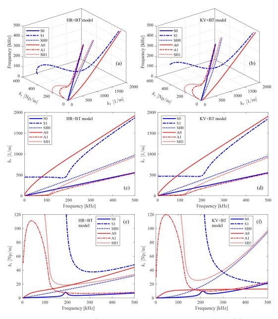
Figure 7.22 – For the unmounted IFS, the predicted dispersion curves at  $\theta = 90^{\circ}$  for HR+BT model (left) and KV+BT model (right): (a) and (b) 3D space of  $(f, k_r, k_i)$ , (c) and (d) projection onto  $(f, k_r)$  plane, (e) and (f) projection onto  $(f, k_i)$  plane.
