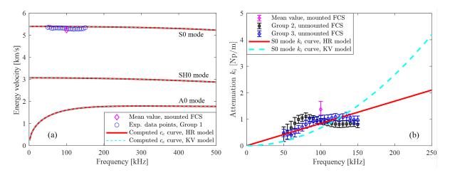
Figure 7.13 – Comparison between the computed and experimentally identified dispersion curves of (a) energy velocity and (b) attenuation coefficient for the unmounted FCS at  $\theta = 0^{\circ}$ .
