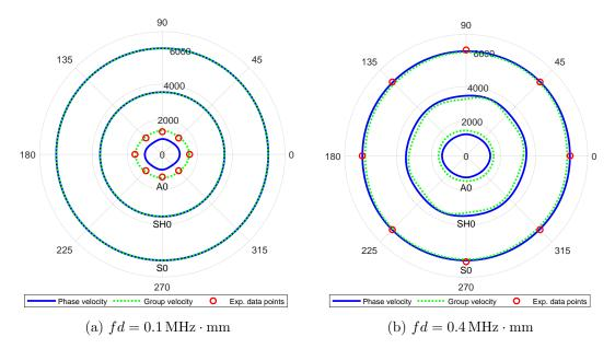
Figure 4.13 – Polar plot of wave velocities. The experimental data points are extracted from [8].
