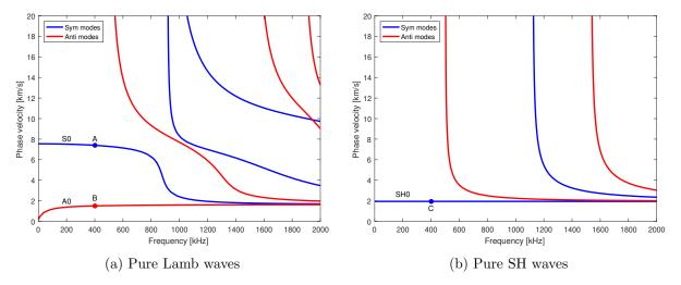
Figure 4.6 – Dispersion curves of pure Lamb and SH waves of the cross-ply laminate when  $\theta = 0^{\circ}$ .
