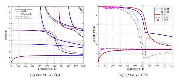
Figure 5.2 – Dispersion curves of Open Guided Waves at the propagation angle  $\theta = 0^{\circ}$  computed via GMM and ESM.
