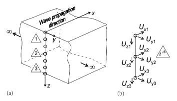
Figure 1.9 – SAFE model of wave propagation, (a) discretization along thickness direction, (b) threenode element and degrees of freedom of each node [7].
