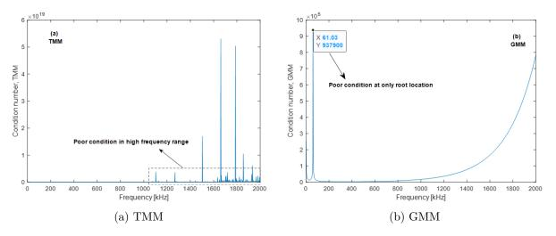
Figure 6.17 – The condition number of matrices of the Open Guided Waves at  $v_0 = 1000$  m/s for (a) the monodromy transfer matrix  $\mathbf{T}^{\text{mono}}$  and (b) the global matrix  $\mathbf{D}_G$ .
