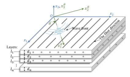
Figure 7.2 – Schematical diagram of a *n*-layered aeronautic composite laminate.
